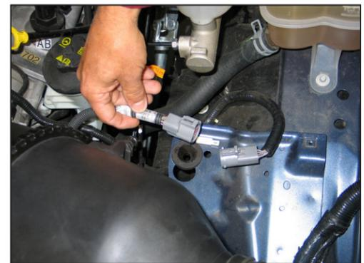
5. Unhook the secondary mass air sensor connection from the clip that secures it to the air box mounting bracket, then disconnect the secondary mass air connection.
