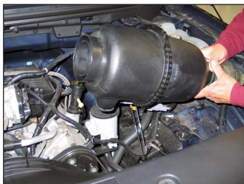
4. Firmly pull up the assembly to unhook it from the mounting grommets and inner fender as shown. **NOTE: Use caution as the mass air sensor electrical harness will still be connected. NOTE: K&N Engineering, Inc., recommends that customers do not discard factory air intake.**
