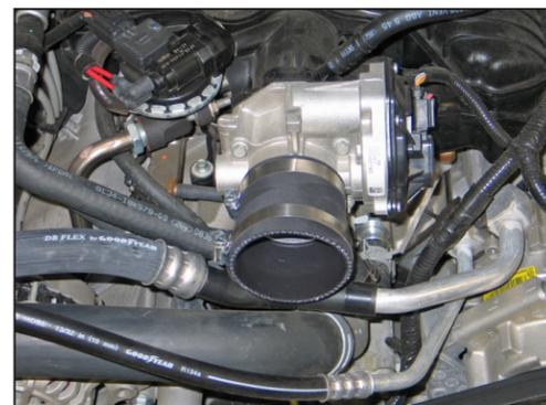
22. Install the silicone hose (08096) onto the throttle body and secure with the provided hose clamp.
