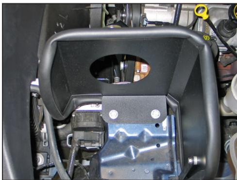
13. Install the heat shield assembly into position with the rubber insert nuts installed into the small portion of the factory holes.
