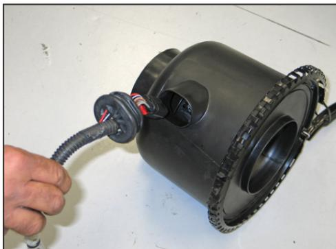
16. Slide the rubber grommet back to gain access to the mass air sensor electrical connector. Using a small screwdriver, release the red locking tab and disconnect the electrical connection, then remove the wiring harness.
