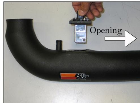
21. Install the mass air sensor assembly into the K&N® intake tube and secure with the provided hardware.
