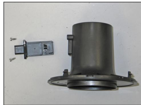
18. Using the supplied T20 TORX, remove the two screws that secure the mass air sensor and then remove the mass air sensor as shown.
