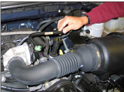
2. Rotate the crank case vent hose locking rings and pull the crank case vent hose off of the valve cover and intake tube as shown.
