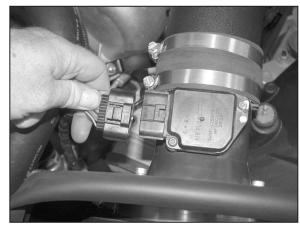
23. Reconnect the mass air sensor electrical connection as shown.
