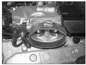
18. Install the provided silicone hose (08623) onto the throttle body and secure with the hose clamp provided.
