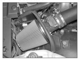
22. Install the mass air filter assembly onto the  $K\&N^{\otimes}$  intake tube and secure with the provided hose clamp.
