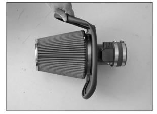
15. Install the K&N® air filter onto the mass air sensor assembly as shown.
