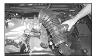
4. Loosen the two hose clamps which secure the stock intake tube to the throttle body and mass air sensor and then remove the intake tube from the vehicle as shown.
