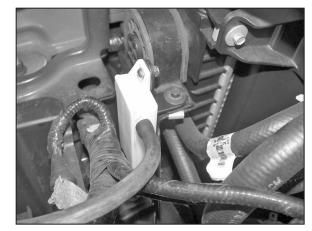
10. Secure the muffler assembly with the bolt removed in step #9 to the radiator mount.
