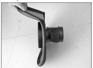
13. Install the radius filter adapter, gaskets and heat shield assembly onto the mass air sensor with the provided hardware as shown.
