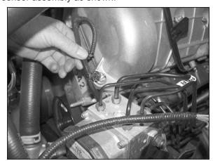
16. Pull up to release the wiring harness clip from valve cover mounting stud.
