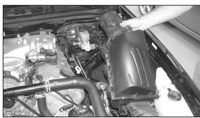
6. Lift and remove the air box from the vehicle as shown.
