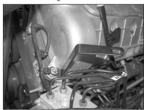
17. Install the tube-mounting bracket (010086) onto the valve cover-mounting stud exposed in step #16 and secure with the provided wire tie to secure the wire harness to the installed bracket.
