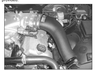
19. Install the K&N® intake tube into the silicone hose at the throttle body and secure with the provided hose clamp.
