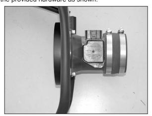
14. Install the silicone hose (08630) onto the mass air sensor and secure with the provided hose clamp as shown.
