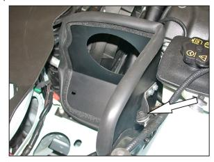
13. Install the heat shield into the vehicle and secure the bracket installed in step #12 to the factory air box mount with the factory bolt removed in step #9.
