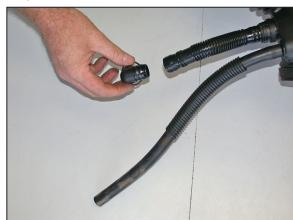
24. Pull firmly on the crank case vent elbow to remove from the vent tube as shown.
