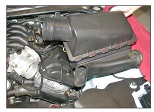
10. Pull up firmly on the air box to dislodge it from the retaining pin, and then remove the air box from the vehicle.
