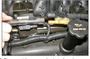
5. Disconnect the evaporative hose from the evaporative valve and cut the two tie wraps securing the hose to the bracket.
