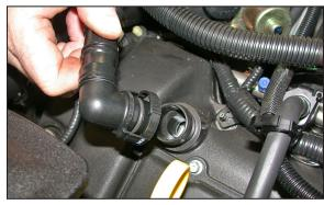
6. Depress the locking ring on the crank case vent hose, and then remove the crank case vent hose from the valve cover.
