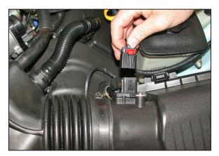
4. Pull back the red locking tab on the mass air sensor electrical connection, and then disconnect the mass air sensor electrical connection.
