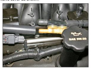
27. Install the supplied 3/8" vent hose onto the K&N® intake tube, and then connect the open end to the evaporative valve as shown.
