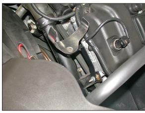
17. Install the saddle bracket assembly onto the threaded stud on the engine as shown and secure with the provided hardware.
