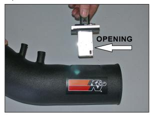
22. Install the mass air assembly into the K&N® intake tube and secure with the provided hardware
