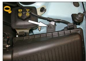
9. Remove the air box retaining bolt shown.
