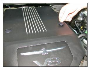
31. Reinstall the engine cover onto the rear retaining clips and then reinstall the retaining clips removed in step #2.
