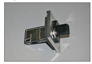
21. Using the screws removed in step #19, install the mass air sensor into the  $K\&N^{\scriptsize @}$  mass air adapter.
