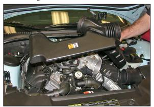
8. Remove the stock intake tube assembly from the vehicle.
