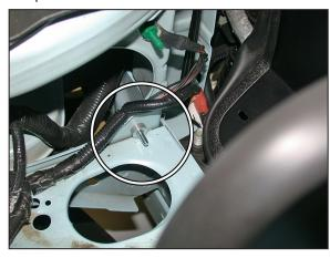
14. Install the provided 6mm bolt through the factory hole in the core support and then install the provided spacer onto the bolt as shown.
