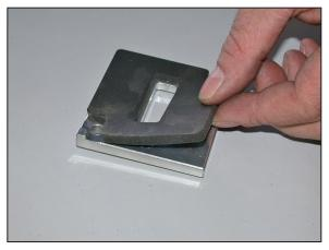
20. Install the provided gasket onto the K&N® mass air adapter as shown.
