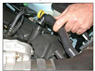
26. Install the vent hose assembly onto the K&N® intake tube and then snap the vent elbow onto the valve cover as shown.
