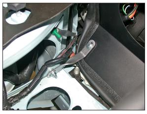
15. Install the provided heat shield bracket (010084) onto the bolt installed in step #14, and then fasten the bracket to the heat shield with the provided hardware.
