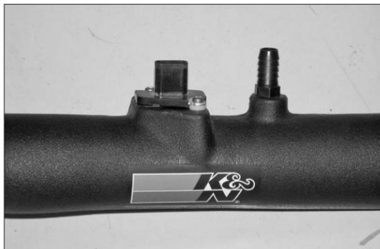
13. Install the vent fitting into the new intake tube as shown.
