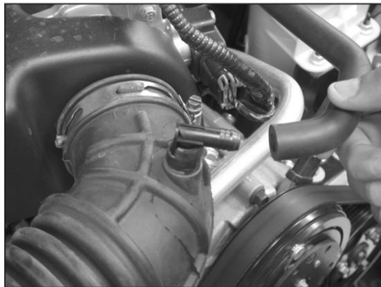
3a. On vehicles equipped with a brake booster breather line, disconnect the breather line from the factory 90° fitting as shown.
