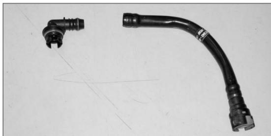
25. Using a razor blade slit the plastic tube and then remove the tube from the valve cover fitting as shown.
