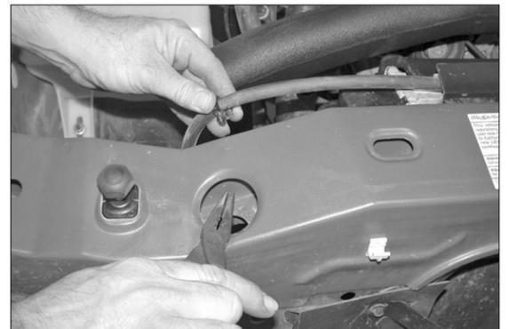
17. Using small pliers, squeeze the cooling system reservoir hose-retaining clip through the large hole in the top of the core support, and then remove the clip from the radiator core support.
