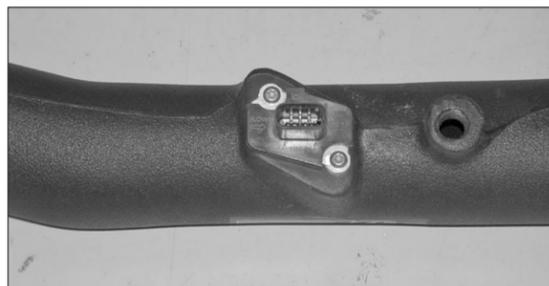
12. Secure the mass air sensor with the factory retaining screws removed in step #8 and spacers provided.
