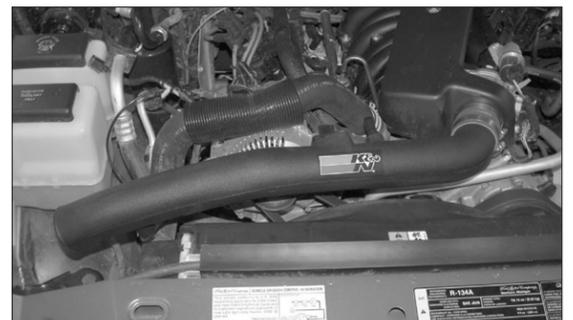
16. Install the intake tube onto the throttle body, then using the bolt removed in step #9 secure the bracket onto the alternator as shown.
