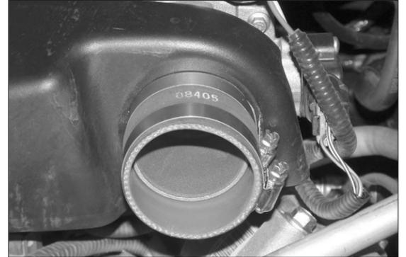
15. Install the provided silicone hose (08405) onto the throttle body as shown.
