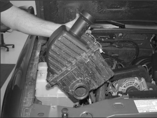
6. Slide a flat blade screwdriver in between the airbox and the airbox mounting tray. Pry downward on the tray, while pulling upwards on the airbox assembly to release the assembly from the retaining grommets in the tray.
