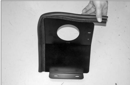
19. Install the edge trim onto the heat shield as shown. Trim if needed.
