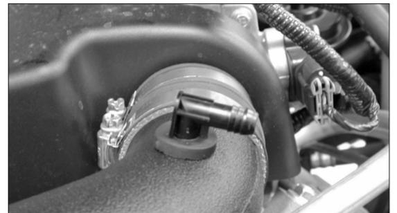
16a. On vehicles equipped with a brake booster breather line, install the factory 90° fitting removed in step #3b into the grommet installed into the K&N® intake tube in step #10b.
