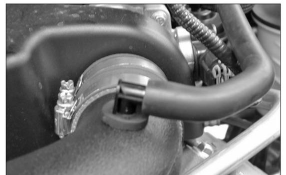
16b. On vehicles equipped with a brake booster breather line, connect the vent line to the 90° fitting installed in step #16a.
