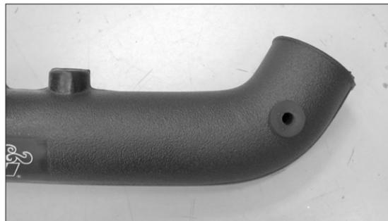
10b. On vehicles equipped with a brake booster breather line, drill a 5/8" id hole into the K&N® intake tube at the location marked in step #10a and install the provided grommet.
