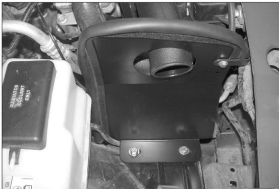
22. Install the heat shield into the vehicle using the 3/8" bolts and washers provided threaded into the inserts installed in step #21.
