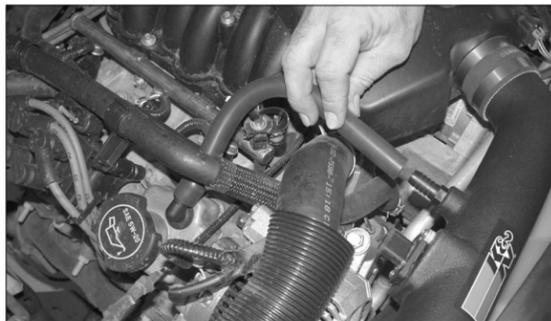
27. Re-install the valve cover fitting into the valve cover and then attach the silicone hose onto the K&N® intake tube as shown.
