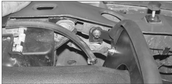
23. Fasten the heat shield mounting bracket to the core support with the bolt and lock washer provided passing through the wiring harness mount into the core support as shown.
