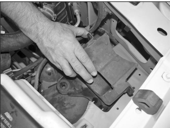
7. Pull firmly on the air inlet duct to release the duct from the radiator core support as shown.
