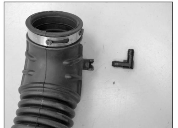
3b. Cut the clamp which secures the 90° fitting to the stock intake hose and then remove the fitting as shown.
