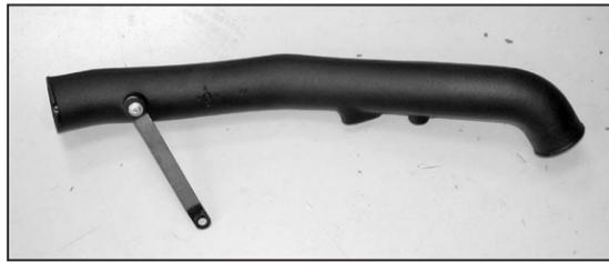
10. Mount the tube-mounting bracket (010078) onto the new K&N® intake tube with the provided hardware as shown.
