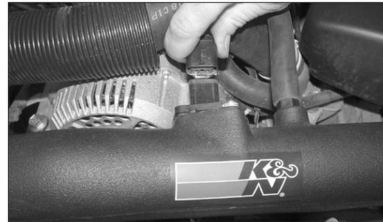
29. Reconnect the mass air electrical connection as shown.
