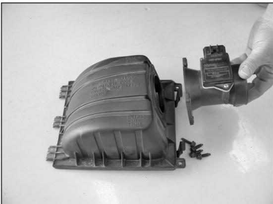
11. Loosen and remove the four hex bolts that secure the mass air sensor, then, remove the mass air sensor from the air box lid.
