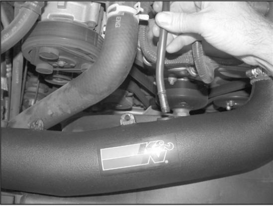
22. Insert the crank case vent into the grommet, as shown.
