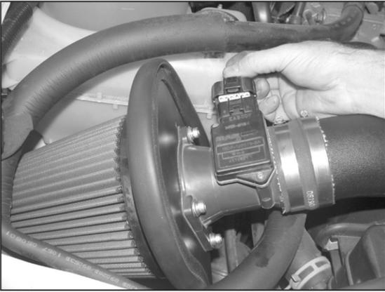
24. Reconnect the mass air sensor electrical connection and secure wire harness in retaining clips onto intake tube.
