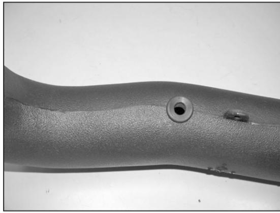
12. Install the crank case vent grommet into the K&N® intake tube as shown.
