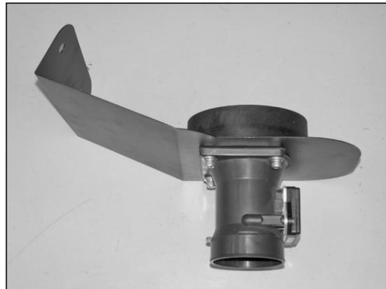
14. Assemble the mass air adaptor, heat shield, gaskets and the mass air sensor as shown using the provided hardware.
