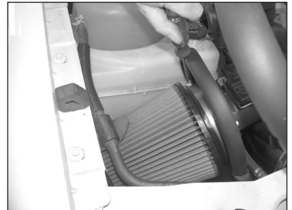
19. Install the K&N® filtercharger onto the mass air assembly as shown.
