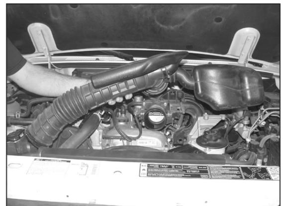
6. Loosen the hose clamps at the throttle body and the mass air sensor, then remove the intake tube as shown.
