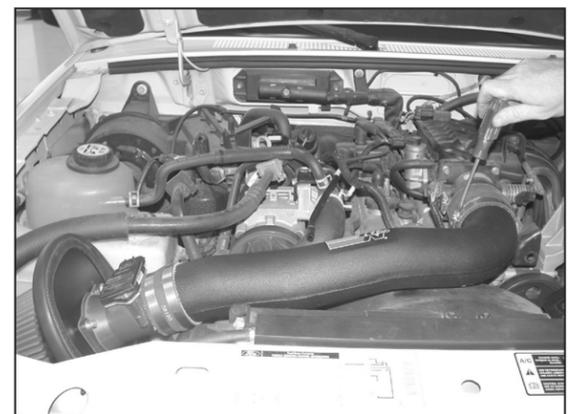
21. Install the K&N® intake tube onto the mass air assembly and then onto the throttle body as shown.
