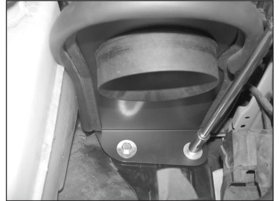
18. Install the mass air assembly onto the air box mounting bracket and secure with the provided 3/8" bolts.
