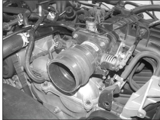
13. Install the provided silicone hose (08696) onto the throttle body with provided hose clamps as shown.
