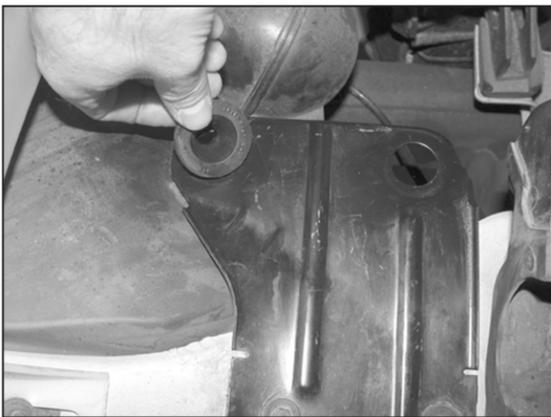
10. Remove the two air box retaining grommets from the air box mounting bracket as shown.
