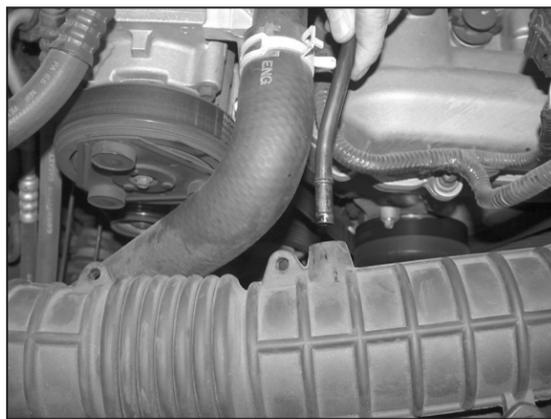
3. Disconnect crank case vent from intake tube as shown.
