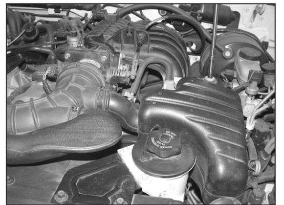
5. Vehicle's equipped with resonator chamber on intake tube, remove the 8mm bolt that secures resonator to mounting bracket.
