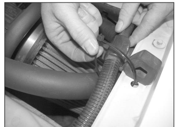
20. Using the provided tie wrap, secure the coolant recovery hose to the inner fender about the K&N® filtercharger.
