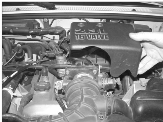
4. Remove the two 7mm screws that secure the throttle body cover then remove the throttle body cover.
