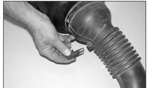
21. Remove the temp sensor from the stock intake tube as shown.
