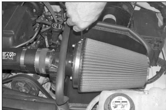
31. Install the Filtercharger onto the mass air sensor and secure it with the provided hose clamp.
