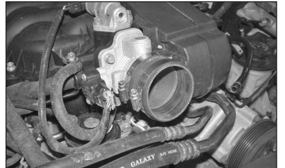
20. Install the provided silicone hose (08756) onto the throttle body with the provided hose clamps.
