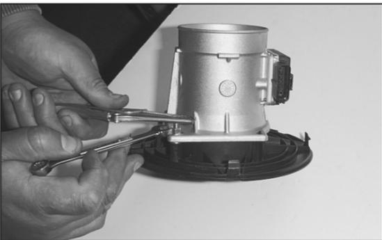
11. Using a pair of small vise grips or pliers, hold the stud while using a 10mm wrench to loosen the nuts, then remove the mass air sensor from the retaining plate.
