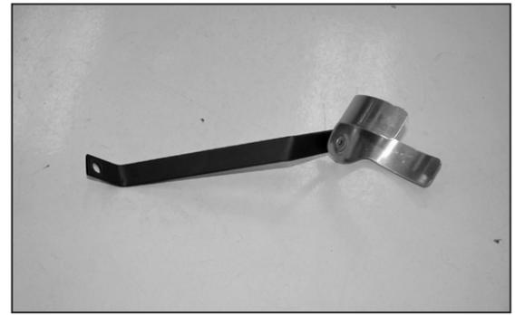
18. On vehicles that did not come equip with A/C, assemble the saddle bracket assembly as shown using bracket (07180).
