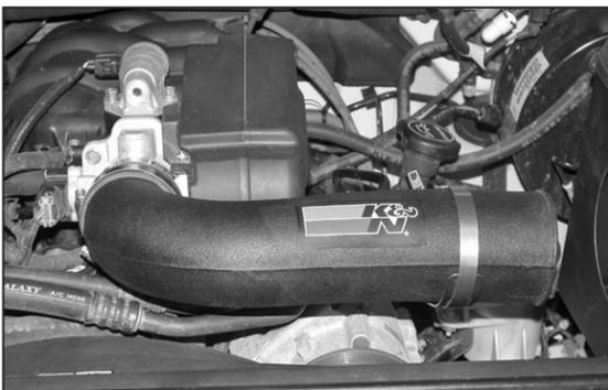
26. Install the K&N® intake tube onto the throttle body, then align with the saddle bracket. Then tighten all hose clamps.
