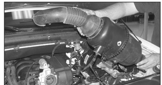
7. Remove the entire stock air intake assembly from the vehicle.
