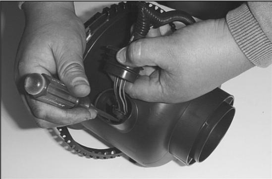
9. Slide the rubber grommet back and disconnect the primary mass air sensor electrical connection, using a flat blade screwdriver.
