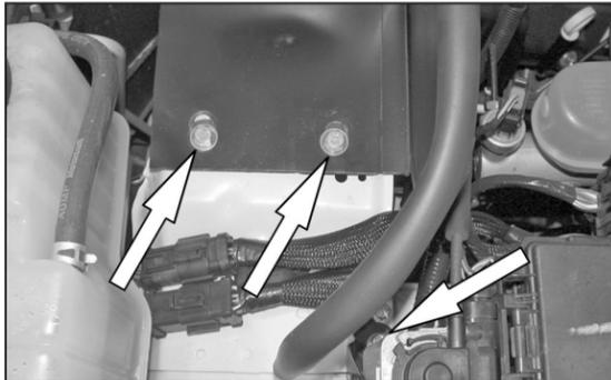
17. On vehicles with cruise control install heat shield as shown with the provided hardware.
