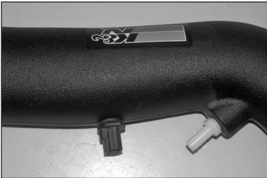
23. Install the temp sensor into the new K&N® intake tube as shown.
