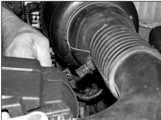
2. Disconnect the air temp sensor electrical connection.
