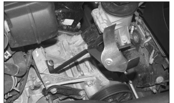
19a. On non A/C vehicles, install the saddle bracket assembly from step 18 onto vehicle with the provided hardware as shown.
