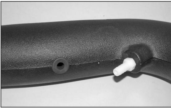
22. Install the provided grommet and vent fitting onto the new K&N® intake tube as shown.
