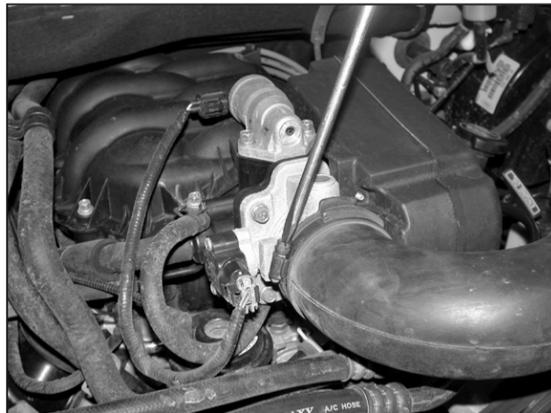
4. Loosen hose clamp at the throttle body.
