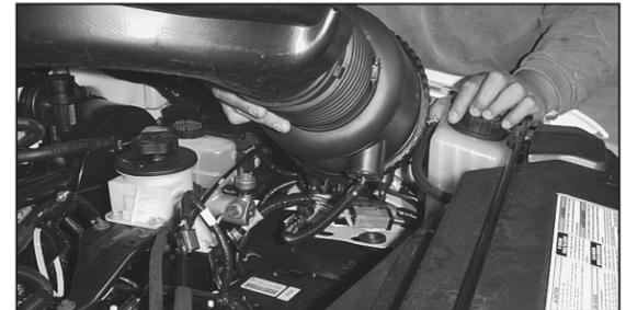
5. Detach the stock intake tube from the throttle body and lift up on the air cleaner assembly to release it from its retaining grommets.
