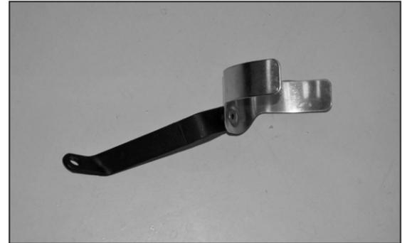
18a. On vehicles that come equip with A/C, assemble the saddle bracket assembly as shown using bracket (07181).
