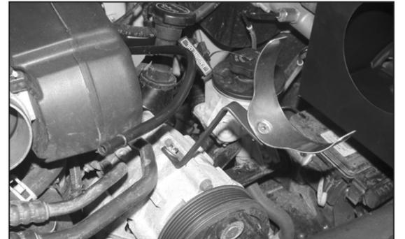
19. On vehicles that come equip with A/C, remove the A/C mounting bolt. Then secure saddle bracket assembly from step 18a onto vehicle with the bolt that was removed.
