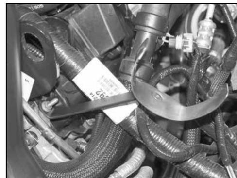
14. Install the saddle bracket assembly onto the engine block and secure with the nut removed in step 12.
