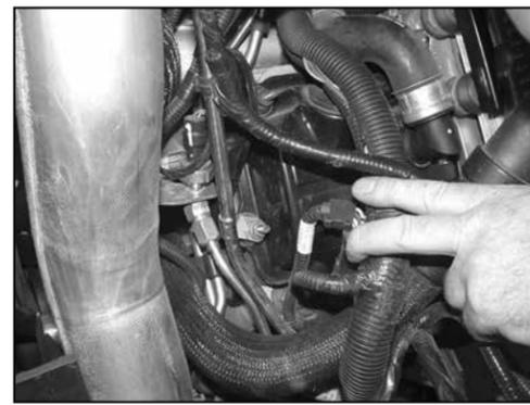
12. Remove the valve cover nut that retains the dip stick to the engine block with a 10mm socket.
