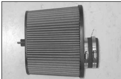
31a. Install the provided silicone hose (08761) onto the air filter flange and secure with the provided hose clamp.
