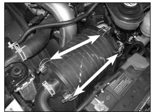
4. Release the four clamps that retain the front and back ends of the air box.
