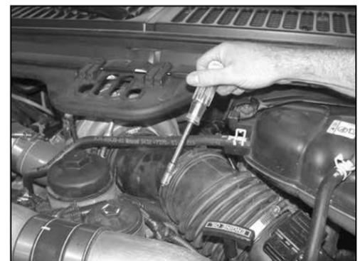
5. On vehicles equipped with a two piece inlet tube and bellows, loosen the hose clamp that secures the turbo inlet tube to the inlet bellows.
