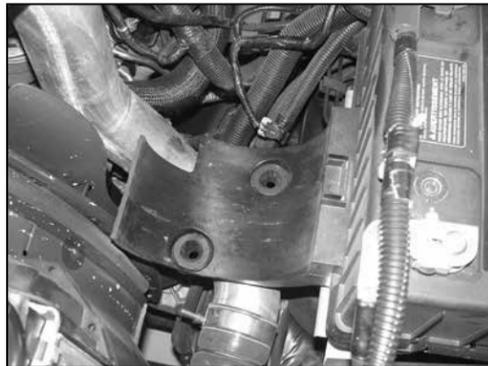
10. Remove the rubber grommets that retain the air box assembly onto the vehicle.
