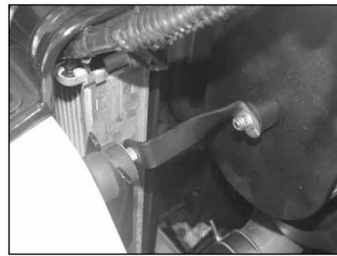
33. Install the provided bracket onto the radiator mount stud and the air filter stud with the provided hardware.
