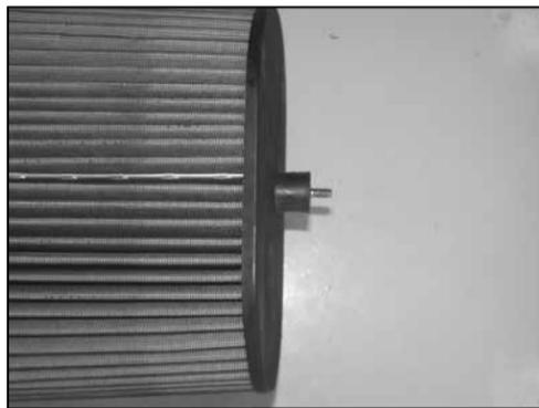
31. Install the provided rubber mounted stud onto the K&N® air filter as shown.
