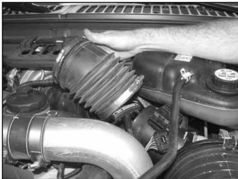
6. On vehicles equipped with a two piece inlet tube and bellows, loosen the hose clamp at the mass air sensor and remove the intake hose from the vehicle.
