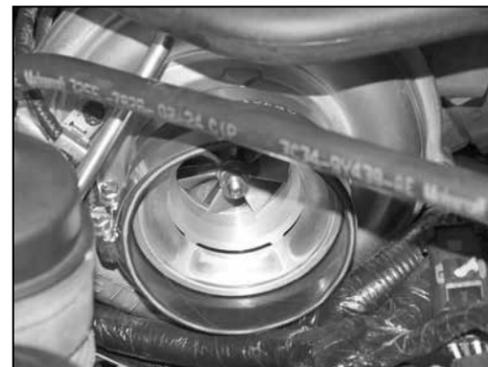
15a. On vehicles equipped with a one piece inlet tube and bellows, install the silicone hose (08761) onto the turbo inlet and secure with the provided hose clamp.
