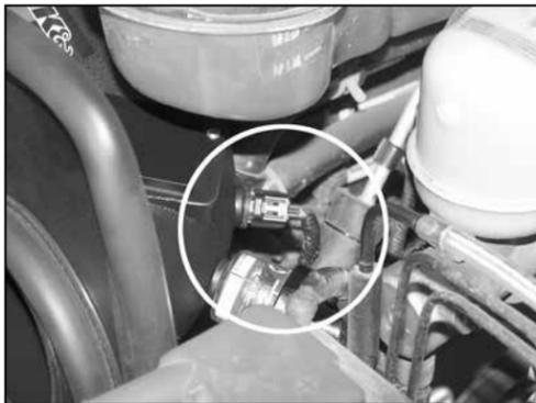
25a. On vehicles equipped with an air temperature sensor, reconnect the air temperature sensor electrical connection as shown.
