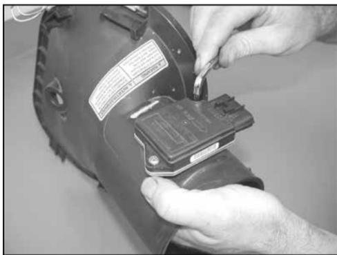
18. On vehicles equipped with a mass air sensor, remove the mass air sensor from the factory air box lid with the provided torx wrench as shown.
