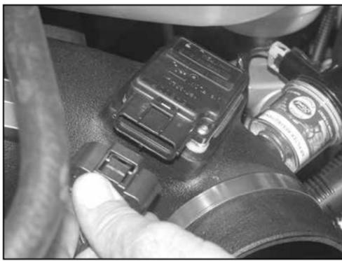
25. On vehicles equipped with a mass air sensor, reconnect the mass air sensor electrical connection as shown.
