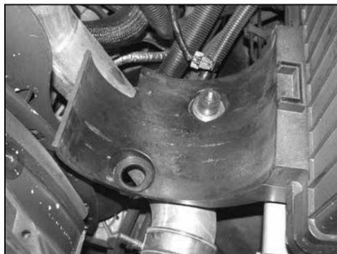
11. Install the rubber mounted stud onto the air box mounting bracket with the provided hardware as shown.
