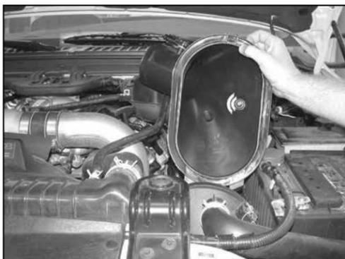
8. Remove the air box base as shown.
