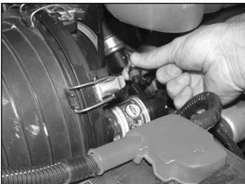
2. Disconnect the restrictor gauge electrical connection as shown.
