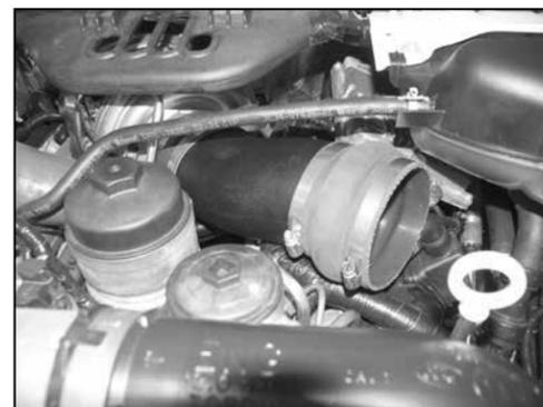
15. On vehicles equipped with a two piece inlet tube and bellows, install the silicone hump hose (08418) onto the stock turbo inlet tube and secure with the provided hose clamp as shown.
