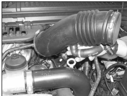
9c. On vehicles equipped with a one piece inlet tube and bellows, remove the inlet bellows and tube assembly from the vehicle as shown.
