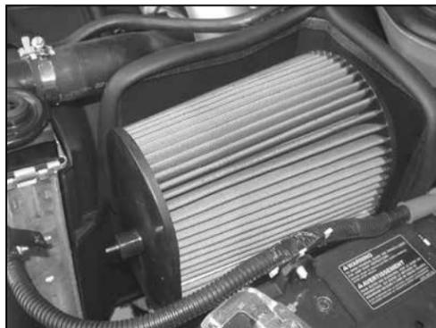
32. Install the air filter element onto the intake tube as shown.
