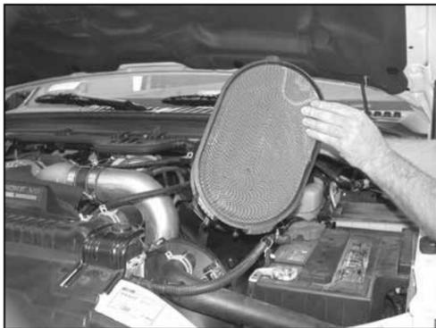
7. Remove the filter housing from vehicle as shown.
