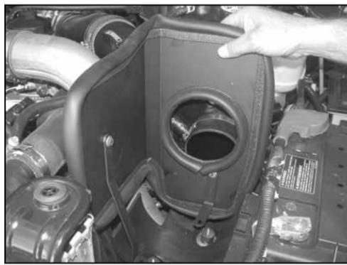
29. Install the heat shield assembly onto the vehicle as shown.
