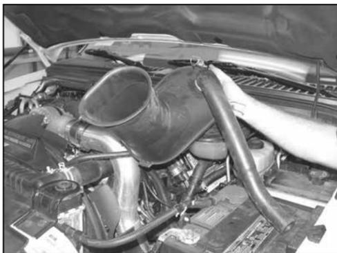
9. Remove the air box top as shown.
