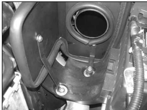
30. Mount the heat shield onto the rubber mounted stud and then secure the long "L" bracket onto the air box mount with the provided bolt and washers.
