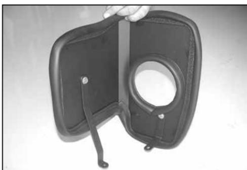
28. Install the two brackets onto the heat shield with the provided hardware as shown. Do not tighten completely.
