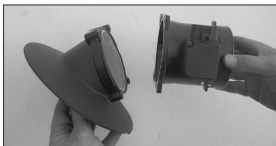
8. Remove the mass air from the air filter housing using a 10mm wrench as shown.
