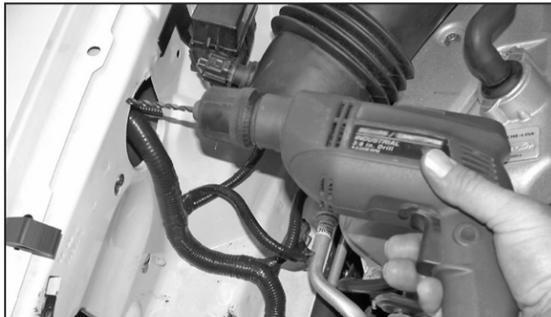
19. Remove the mass air assembly from the vehicle and using a 3/16 drill bit, drill out the marks.
