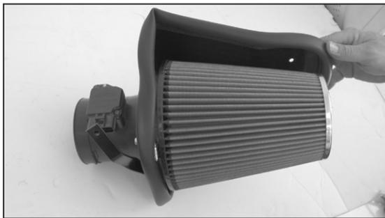
21. Install the filter charger onto the mass air assembly and secure it with the provided hose clamp.
