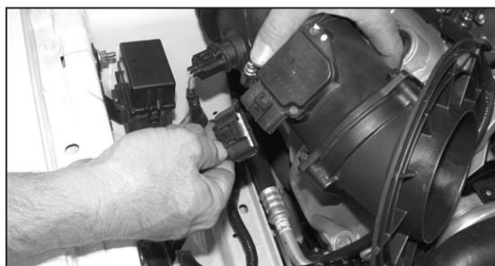
6. Disconnect the mass air electrical connection.
