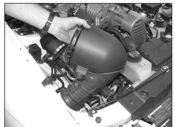
10. Pull the air filter assembly upward and remove from vehicle.
