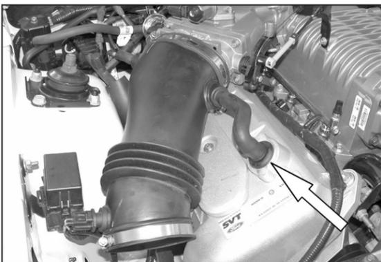
15. Reconnect the intake tube onto the throttle body then reconnect the crank case vent.
