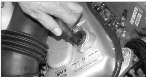
4. Remove crank case vent hose from valve cover as shown.
