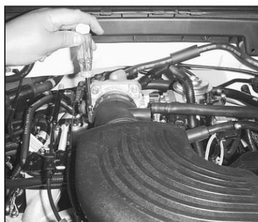
5. Loosen the hose clamp on the stock intake tube at the throttle body.
