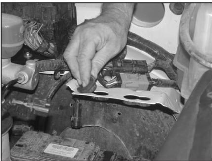
13. Remove the two air box mounting grommets from vehicle as shown.
