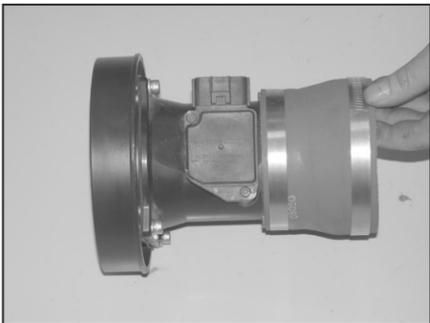
28. Install the silicone hose (#08050) onto the mass air sensor with the provided hardware as shown.
