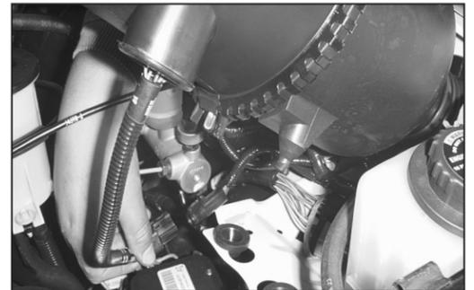
7. Disconnect the secondary mass air sensor electrical connection.
