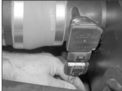
30. Reconnect the primary and secondary mass air electrical connections.
