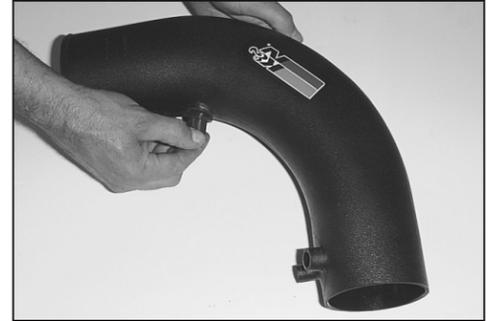
20. Using the provided grommet, install the air temperature sensor into the K&N® intake tube.
