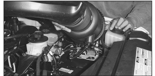
6. Detach the stock intake tube from the throttle body and lift up on the air cleaner assembly to release it from its retaining grommets.
