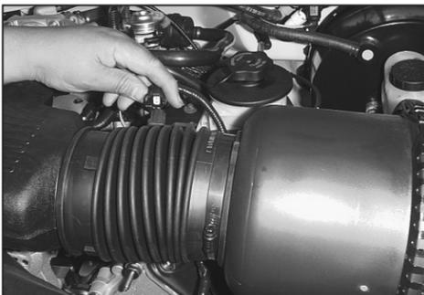
3. Disconnect the air temperature sensor electrical connection.
