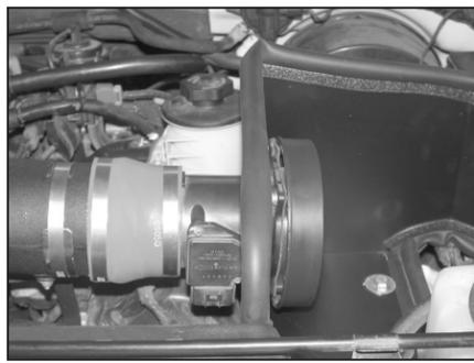
29. Attach the mass air assembly to the intake tube. Secure the mass air assembly and saddle bracket to the intake tube using the provided hose clamps.
