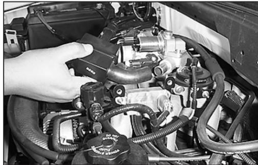
4a. On models with 4.6L engines, detach the air bypass valve and crank case vent hose from the stock intake tube.
