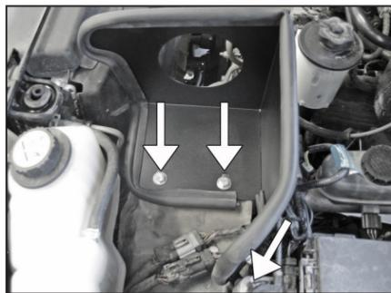
18. On vehicles equipped with cruise control, set the heat shield into position on the air filter mounting bracket. Then secure the heat shield with the provided hardware as shown.
