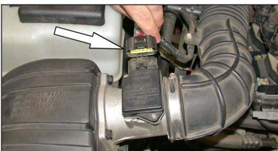
3. Disconnect the mass air electrical connection as shown.
