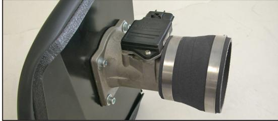
18. Install the silicone hose (08724) onto the mass air sensor with the provided hose clamps.
