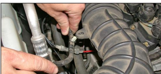
4. Disconnect the mass air wiring loom from the intake tube as shown.
