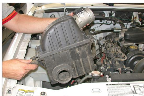
7. Using a screwdriver, pry up the bottom of the air cleaner to release from the stock grommets, then remove the air cleaner assembly as shown.
