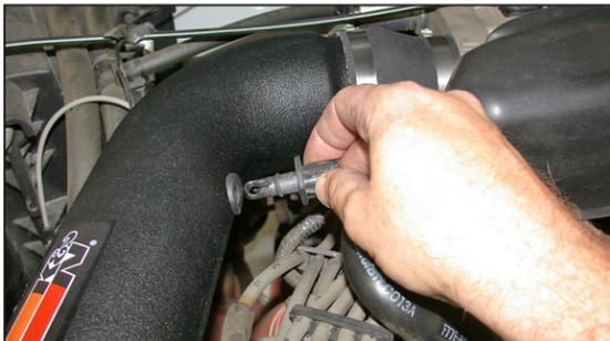
22. Install the temp sensor into the new K&N® intake tube as shown.
