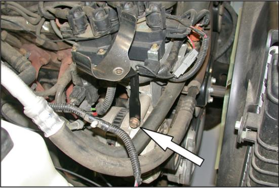
12. Install the saddle bracket assembly onto the alternator with the bolt that was removed in the previous step.
