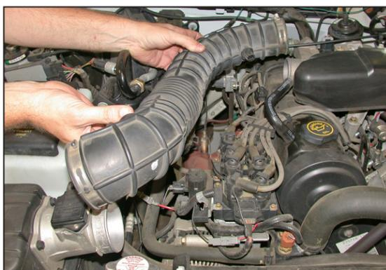
6. Remove the intake tube as shown.
