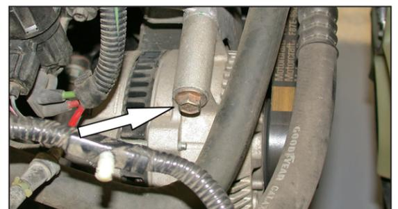
11. Remove the bolt, with a 13mm wrench, that retains the alternator onto the motor.
