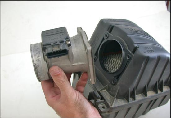
15. Remove the 4 bolts, with a 10mm socket, that secure the mass air onto the airbox, then remove mass air as shown.
