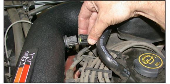
23. Reconnect the air temp electrical connection as shown.
