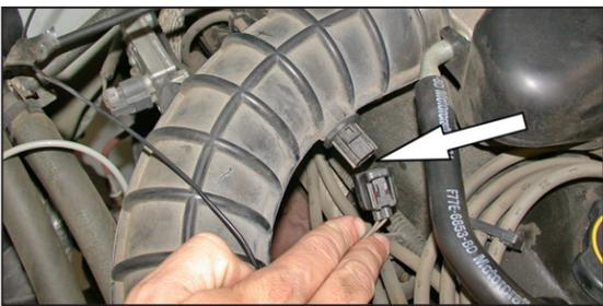
2. Disconnect the air temp. electrical connection.
