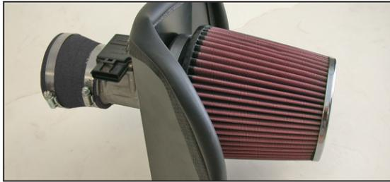
19. Install the K&N® Filtercharger onto the mass air assembly as shown.
