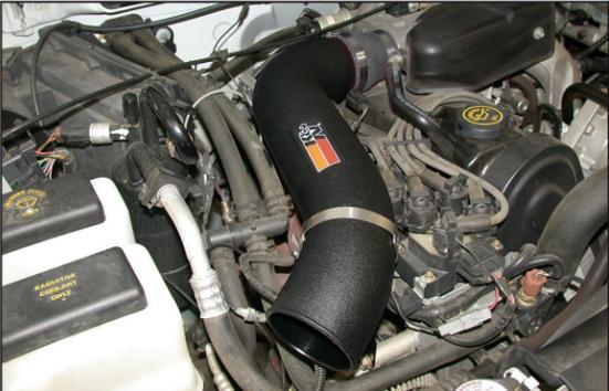
14. Install the new K&N® intake tube onto the throttle body and saddle bracket with the provided hose clamps.
