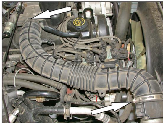
5. Loosen the two hose clamps at the throttle body and the airbox.
