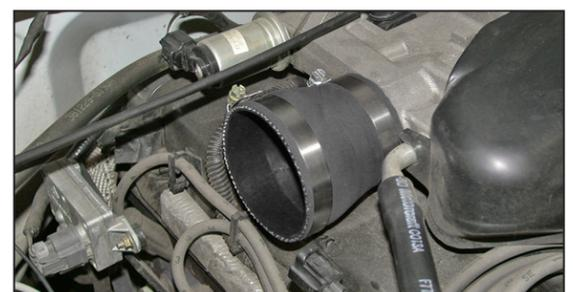
9. Install the provided silicone hose (08713) onto the throttle body with the provided hose clamps.
