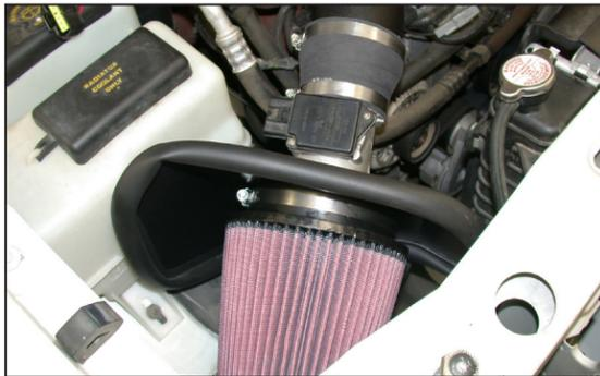
20. Install the mass air assembly onto the new K&N® intake tube then properly position the heat shield assembly into the vehicle and tighten the hose clamps at the throttle body and saddle bracket.
