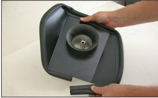
17. Install the edge trim onto the heat shield as shown. Trim if necessary.
