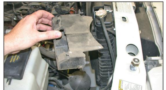
8. Remove the fresh air duct from vehicle.
