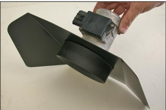
16. Assemble the heat shield and filter adapter onto the mass air sensor with the provided hardware and gasket.
