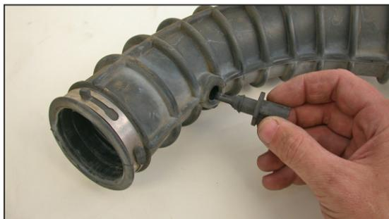
21. Remove the air temp sensor from the stock intake tube as shown.
