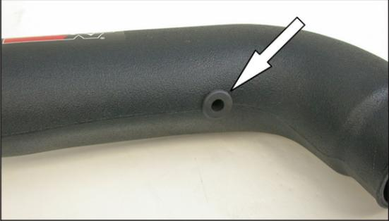
13. Install the provided rubber grommet onto the new K&N® intake tube as shown.
