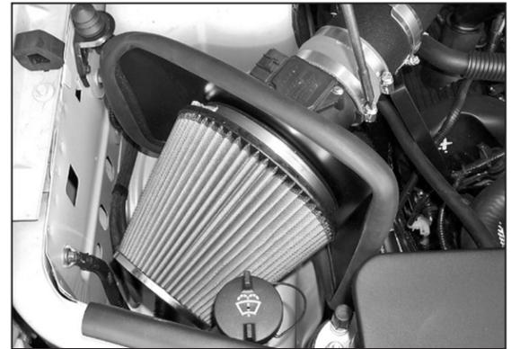
21. Install the heat shield assembly onto the K&N® intake tube and tighten the hose clamp as shown. **NOTE: Adjust heat shield for best clearance before tightening.**
