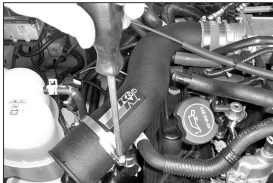
17. Secure the intake tube to the saddle bracket assembly with the provided hose clamp.
