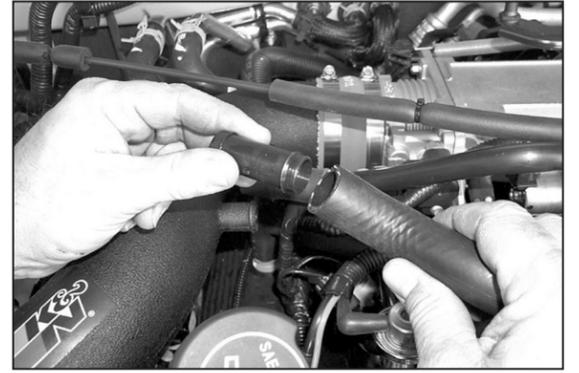
18. Remove the factory hose mender from vent hose as shown.
