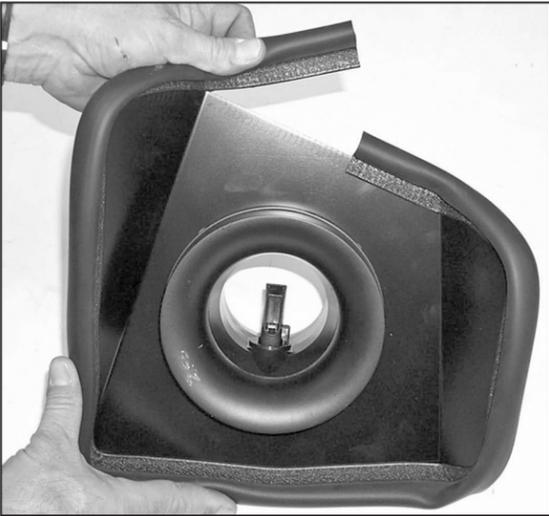
9. Apply the trim seal to the heat shield assembly as shown. Trim if needed.
