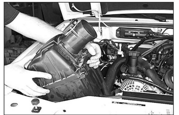
6. Using a screwdriver, pry up the bottom of the air cleaner to release the air cleaner from the stock grommets, then remove the air cleaner assembly as shown.
