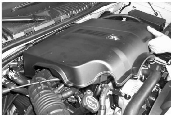
3. Loosen and remove the two 11mm nuts that secure the engine cover, then remove the cover as shown.
