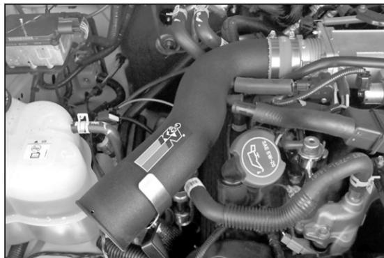
16. Install the K&N® intake tube onto the throttle body then line it up with the saddle bracket assembly as shown.
