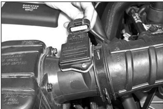
2. Disconnect the mass air sensor electrical connection.
