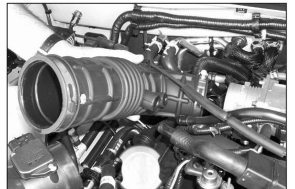
5. Loosen the hose clamp at the throttle body and at the mass air sensor, then remove the stock air intake tube as shown.
