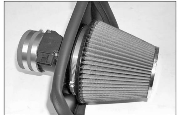
20. Install the K&N® air filter onto the heat shield assembly as shown.
