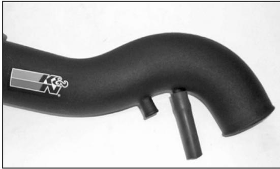
15. Install the silicone hose onto the K&N® intake tube as shown.
