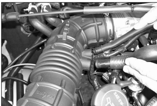
4. Remove the crankcase vent hose and idle bypass hose and cruise control cable from the stock intake tube as shown.
