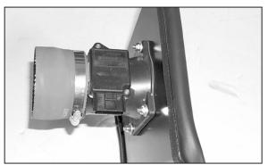
11. Assemble the silicone step hose (08051) and the hose clamps onto the heat shield assembly.
