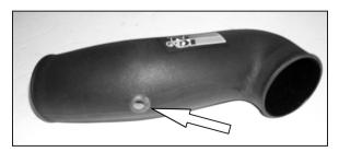
15. Install the provided grommet into the new K&N® intake tube as shown.
