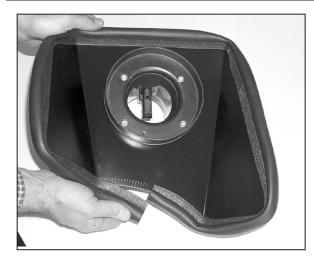
10. Apply the trim seal to the heat shield assembly as shown. Trim if needed.
