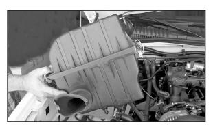
7. Using a screwdriver, pry up the bottom of the air cleaner to release the air cleaner from the stock grommets, then remove the air cleaner assembly as shown
