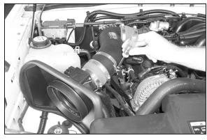
17. Install the K&N® intake tube and heat shield assembly onto the throttle body then secure the intake tube to the saddle bracket assembly with the provided hose clamp.
