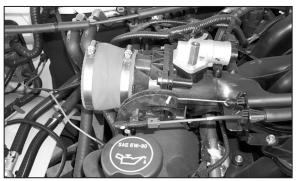
12. Install the silicone step hose (08050) and hose clamps onto the throttle body as shown.
