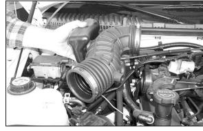
6. Loosen the hose clamp at the throttle body and at the mass air sensor, then remove the stock intake tube as shown.
