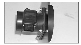
9. Assemble the mass air adapter, gaskets, heat shield and mass air sensor as shown.
