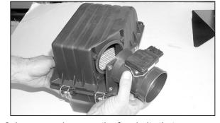
8. Loosen and remove the four bolts that secure the mass air sensor, then remove the mass air sensor as shown.
