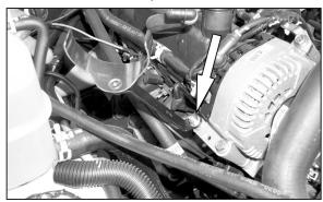
14. Install the saddle bracket assembly onto the alternator mounting stud with the provided 8mm nut and washer.
