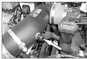
18. Re-connect the crankcase vent hose to the K&N® intake tube as shown.
