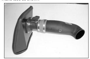
16. Install the rubber hose onto the K&N® intake tube as shown.
