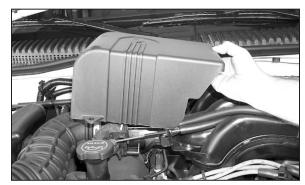
4. Loosen the two T25 torx screws that secure the throttle body cover then remove the cover as shown.
