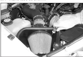
19. Install the K&N® Filtercharger onto the mass air adapter and secure it with the provided hose
