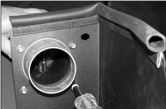
13. Slide the mass air assembly into the bolt pattern on the heat shield, then, secure it with the provided hardware as shown.
