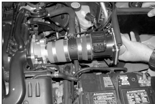
20. Install the K&N® intake assembly onto the throttle body as shown.
