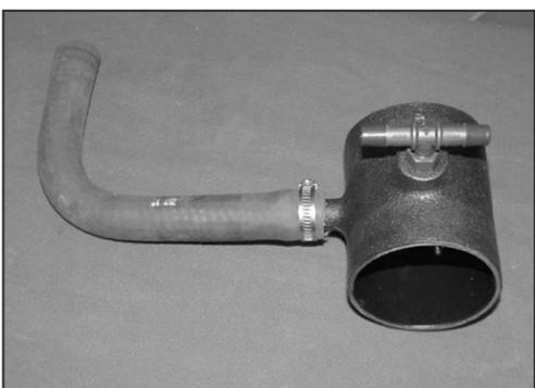
15. Install the provided hose and hose clamp onto the K&N® intake tube as shown.
