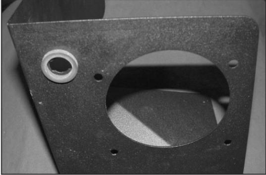
11. Apply the provided adhesive back gasket to the key-hole on the heat shield as shown.
