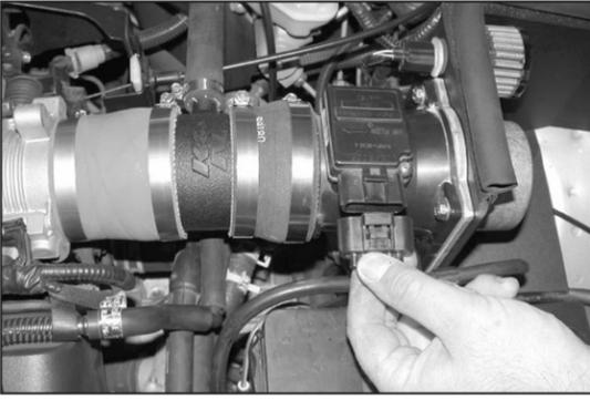
28. Reconnect the mass air sensor electrical connection as shown.
