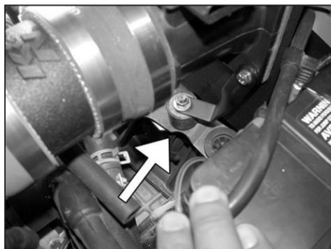
21. Line up the twist bracket with the rubber mounted stud, and secure it with the provided hardware as shown.
