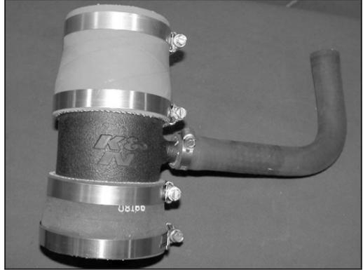
17. Assemble the small silicone step hose and hose clamps onto the K&N® intake tube as shown.
