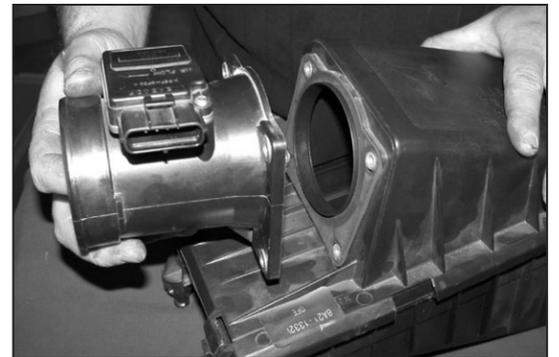
9. Loosen and remove the four bolts that secure the mass air sensor to the air cleaner, then, remove the mass air sensor as shown.
