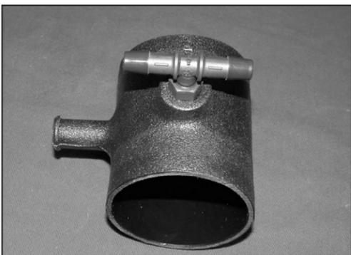
14. Install the provided "T" vent into the threaded boss on the K&N® intake tube as shown.
