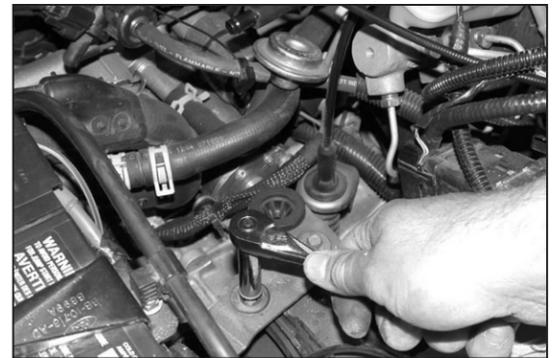
7. Loosen and remove the stock hex bolt from the air cleaner support bracket as shown.
