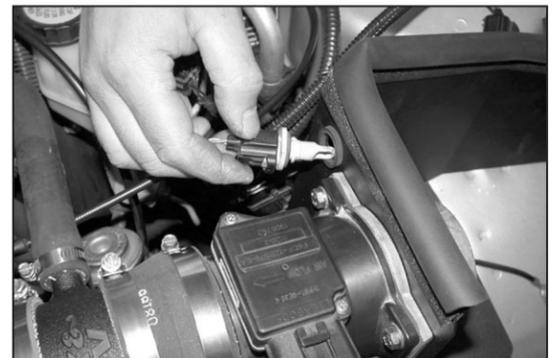
26. Install the air temperature sensor into the key-hole in the heat shield as shown. Turn it ¼ turn to lock into place.
