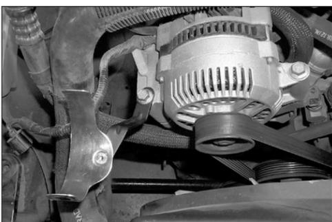
16. Using the bolt removed in step 9, secure the saddle bracket assembly to the alternator as shown. Do not tighten completely at this time.
