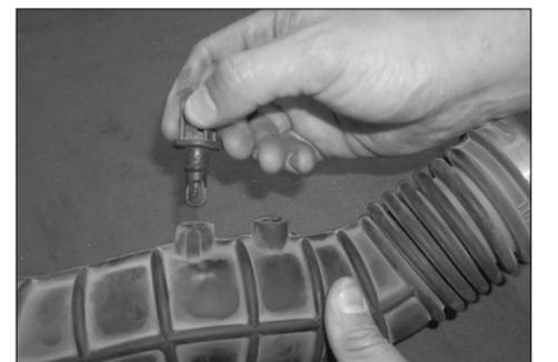
10. Remove the air temperature sensor from the stock rubber intake tube as shown.
