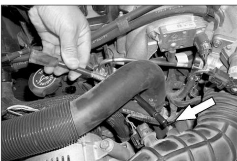
4. Disconnect and remove the crank case vent hose from the stock rubber intake tube as shown.
