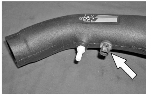
20. On vehicles equipped with an air temperature sensor, install the provided rubber grommet into the hole on the K&N® intake tube, then push the stock air temperature sensor into the grommet as shown. **NOTE: Take care when handling the temp sensor as it is very fragile.**
