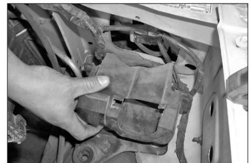
8. Pull firmly on the air inlet duct to release the duct from the radiator core support as shown. **NOTE: K&N Engineering, Inc., recommends that customers do not discard factory air intake.**
