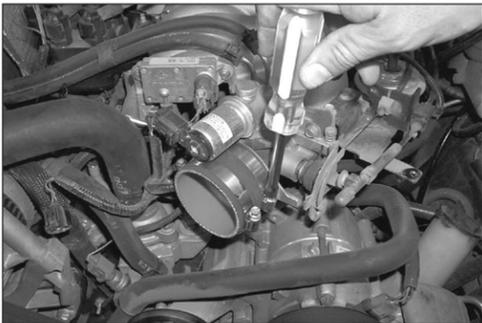
14. Install the silicone hose and hose clamps onto the throttle body as shown.
