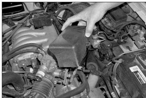
5. Loosen and remove the two bolts that secure the throttle linkage cover then remove the cover as shown.
