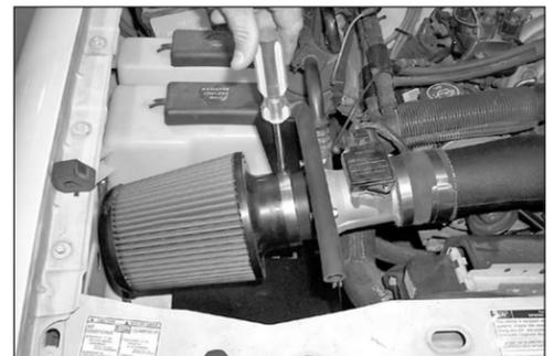
27. Install the K&N® air filter and secure with the provided hose clamp.
