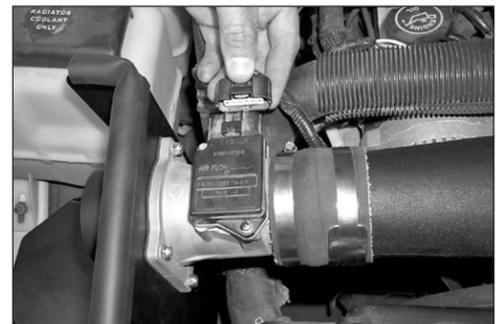
26. Reconnect the mass air sensor electrical connection as shown.
