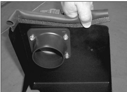
13. Install the trim seal onto the top edge of the heat shield assembly as shown
