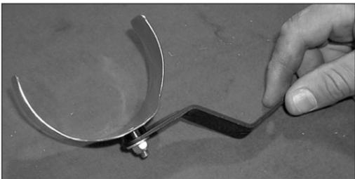
15. Assemble the saddle bracket assembly using the provided hardware as shown.
