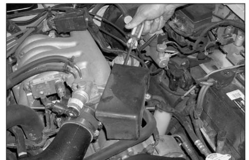
28. Install the stock throttle linkage cover using the factory bolts removed in step 5.
