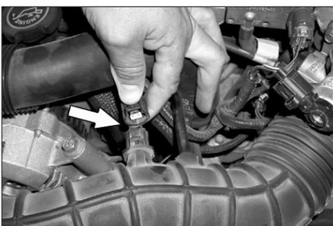
3. On vehicles equipped with an air temperature sensor disconnect the electrical connection as shown.
