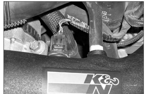
25. Reconnect the air temperature sensor electrical connection as shown.
