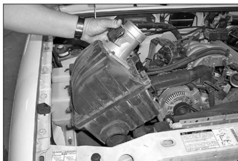
7. Slide a flat blade screwdriver in between the air cleaner and the air cleaner mounting tray. Pry downwards on the tray, while pulling upwards on the air cleaner assembly to release the assembly from the retaining grommets in the tray.
