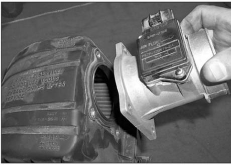
11. Loosen and remove the four hex bolts that secure the mass air sensor, then remove the mass air sensor from the air cleaner as shown.
