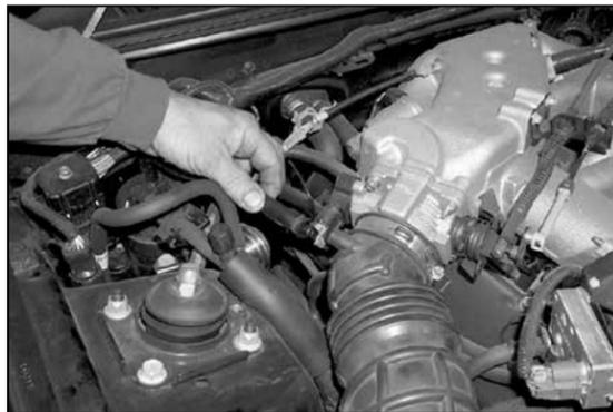
4. Disconnect the crank case vent hose from the rubber intake as shown.
