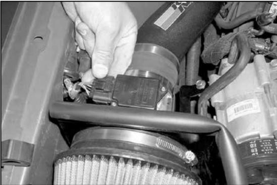
28. Reconnect the vehicles mass air sensor electrical connection as shown.
