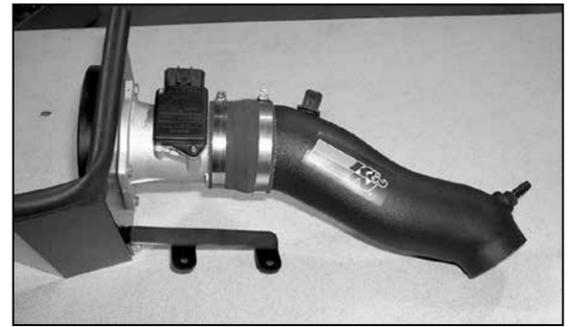
21. Slide the K&N intake tube onto the mass air sensor as shown, but do not tighten completely.
