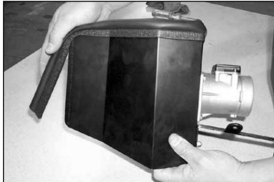
16. Install the provided trim seal onto the heat shield assembly as shown. Trim excess if necessary using side cutters.
