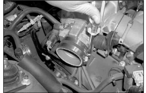
22. Install the provided silicone hose and hose clamps onto the throttle body as shown.
