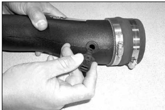
18. On 1999-2000 vehicles install the provided grommet into the hole on the K&N intake tube, then, install the air temperature sensor into the grommet as shown.
