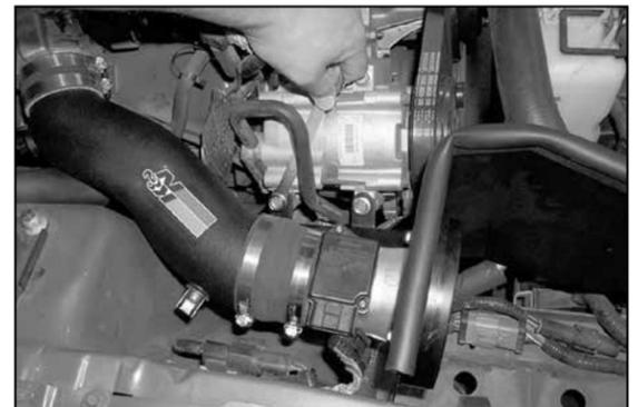
24. Line up the support bracket with the A/C compressor and secure with the original bolts removed in step 13 using a 13mm wrench.
