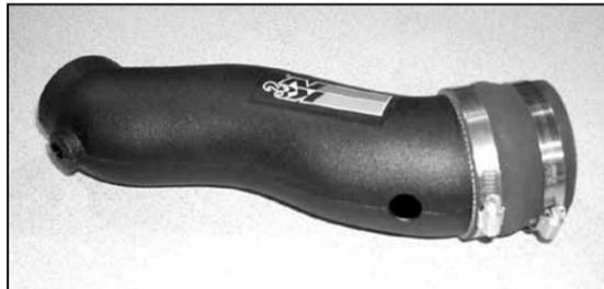
17. Install the provided silicone hose and hose clamps onto the K&N intake tube as shown.
