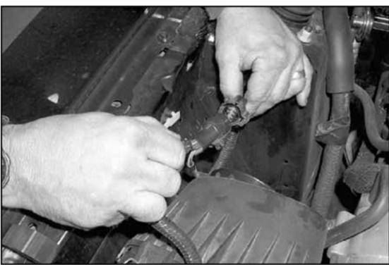
2. Disconnect the secondary mass air sensor electrical connection as shown.
