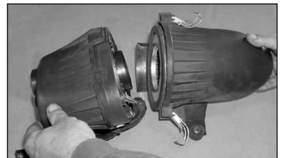
8. Release the over-center clamps on the air cleaner to separate the two halves as shown.
