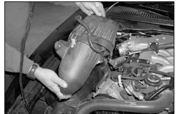
7. Pull firmly upwards to release the air cleaner from the factory grommets, then remove the air cleaner as shown.
