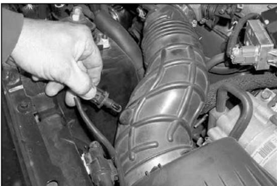
3. On 1999-2000 vehicles remove the air temperature sensor from the rubber intake as shown.
