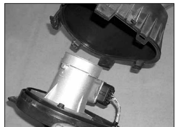
9. Using a flat blade screwdriver, depress the tabs to release the mass air sensor cover from the mass air sensor base plate as shown.
