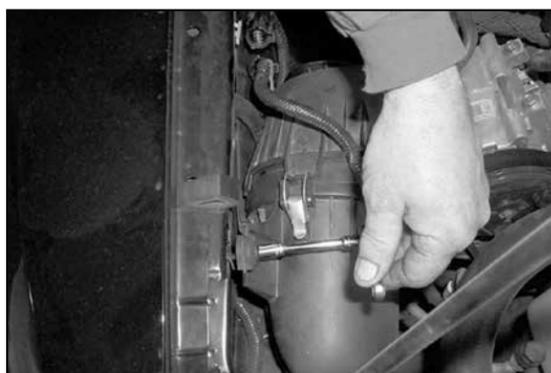
6. Using a 8mm wrench or nut driver, loosen and remove the bolt that secures the air cleaner to the inner fender as shown.
