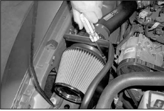
26. Install the K&N® Air filter and secure with the provided hose clamp as shown. Adjust intake tube and tighten all clamps completely.
