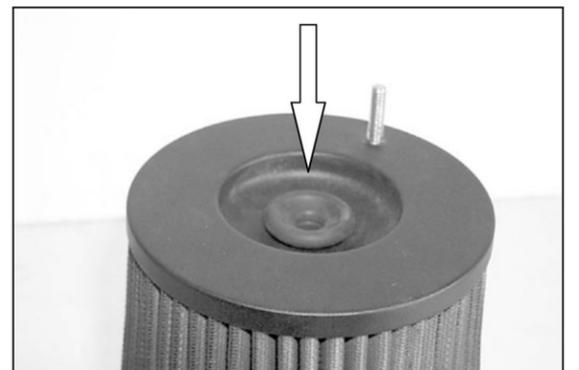
25. Install the grommet that was removed in step 24 into the hole on the top of the K&N® air filter as shown
