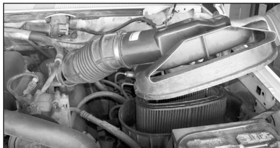
4. Loosen the hose clamp at the turbo inlet tube, then remove the upper air cleaner assembly as shown.
