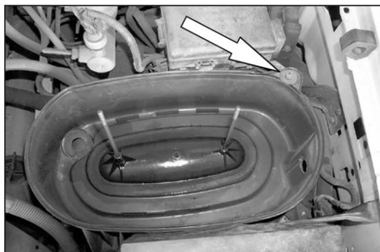
6. Loosen the nut that secures the lower air cleaner assembly as shown.
