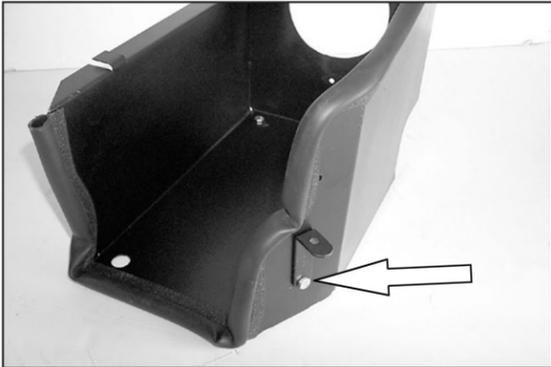
11. Using the provided hardware, install the large "L" bracket onto the K&N® heat shield as shown.
