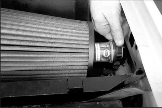
28. Install the Filter minder into the grommet on the end of the filter as shown.
