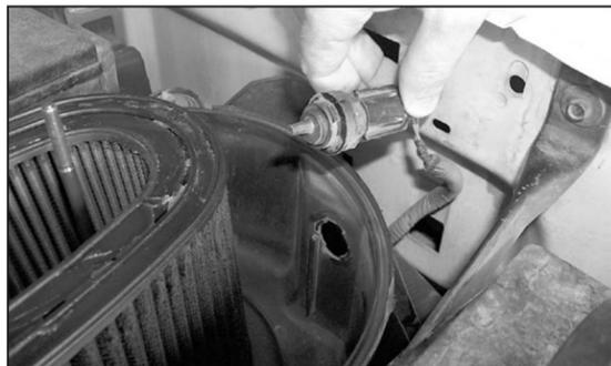
5. To remove the air temperature sensor, turn the sensor 1/4 turn, then, pull the sensor out of the lower air cleaner assembly as shown.
