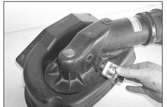
24. Remove the stock filter minder and the stock grommet from the stock air cleaner top as shown.
