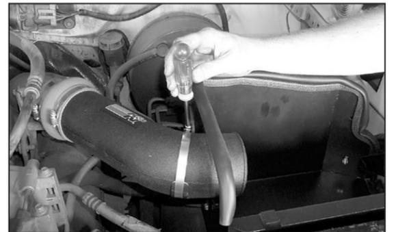
23. Secure the K&N® intake tube to the saddle bracket with the provided hose clamp as shown.
