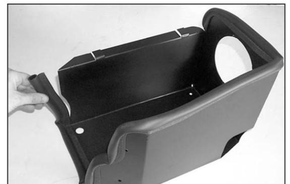
9. Apply the provided trim seal to the K&N® heat shield as shown.
