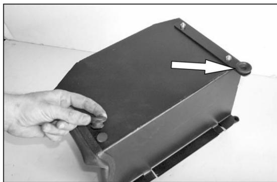
18. Install the stock rubber grommets from the lower air cleaner assembly into the K&N® heat shield assembly as shown.
