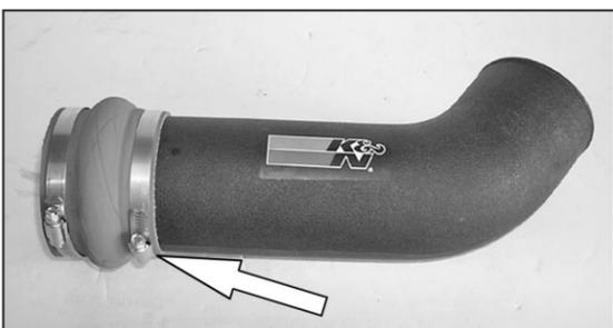
14. Install the silicone hump hose onto the K&N® intake tube as shown and secure with the provided hose clamp.
