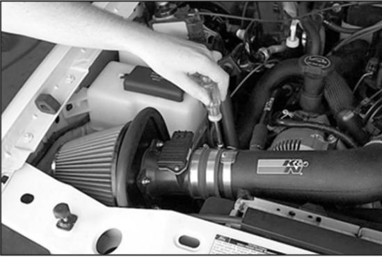
23. Install the heat shield assembly onto the K&N® intake tube and tighten the hose clamp as shown.
