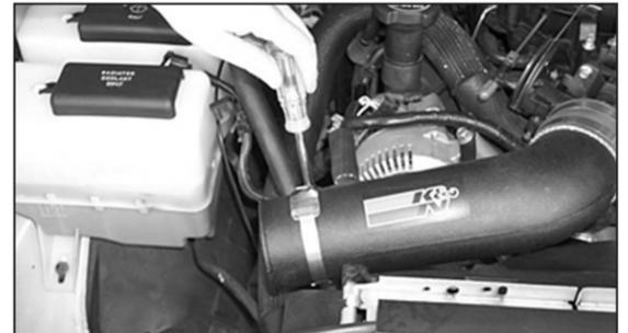
19. Re-install the K&N intake tube onto the throttle body then secure the intake tube to the saddle bracket assembly with the provided hose clamp.
