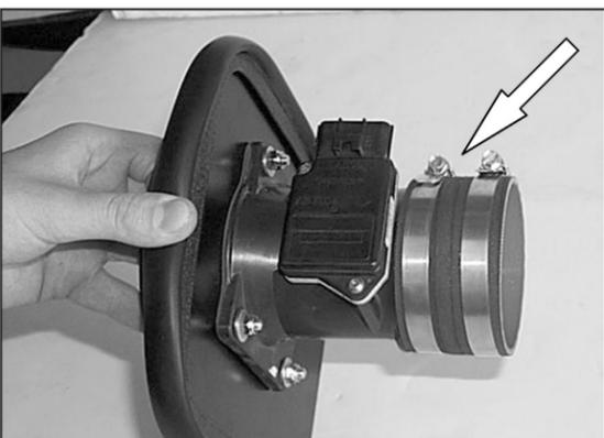
11. Assemble the silicone hose and the hose clamps onto the heat shield assembly as shown.
