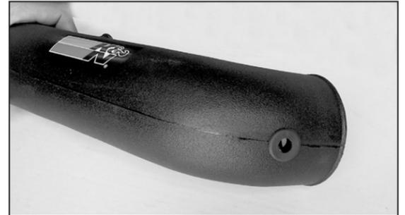
18a. After marking the intake tube, remove the tube from the vehicle and drill a 5/8" hole into the intake tube then install the provided grommet as shown.
