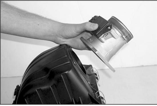
7. Loosen and remove the 4 bolts that secure the mass air sensor then remove the mass air sensor as shown.
