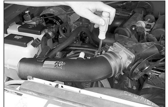
19. Install the K&N® intake tube onto the throttle body as shown.
