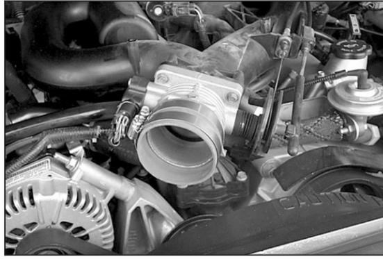
12. Install the silicone hose and hose clamps onto the throttle body as shown.
