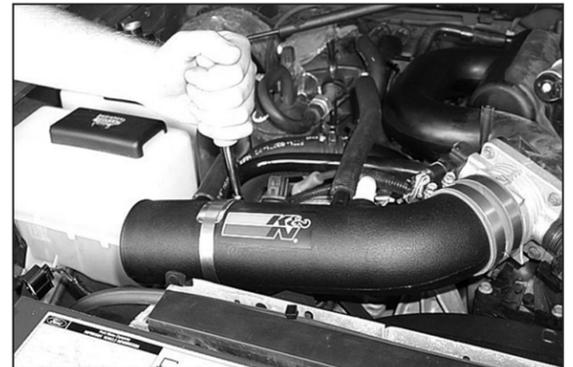
20. Secure the K&N® intake tube to the saddle bracket assembly with the provided hose clamp as shown.
