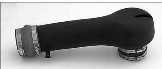
15. Install the silicone hump hose onto the new intake tube.
