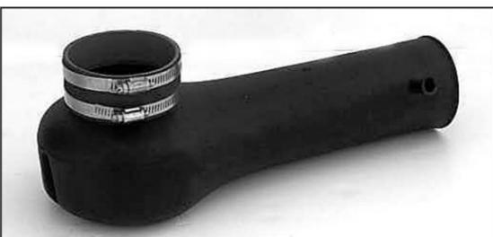
14. Install the silicone hose onto the new intake tube.
