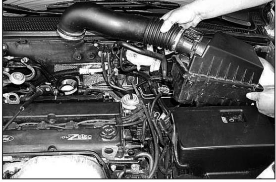
5. Pull firmly up on the air box to release from mounting grommets, and then remove the entire assembly.
