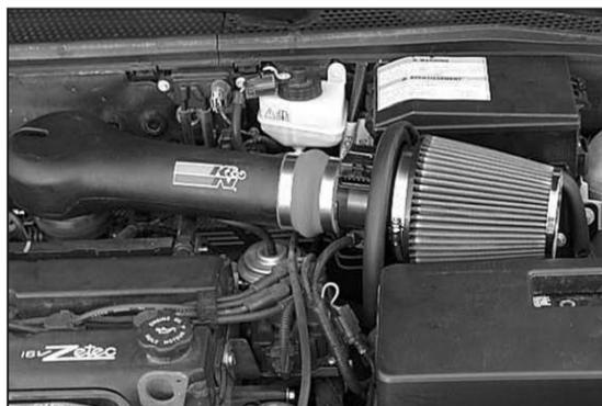
20. Install the filter onto the mass air adapter, then tighten the clamp.
