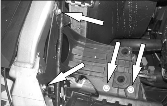
10a. On 2004 and later vehicles loosen and remove the four bolts, which retain the air box-evaP canister bracket shown.
