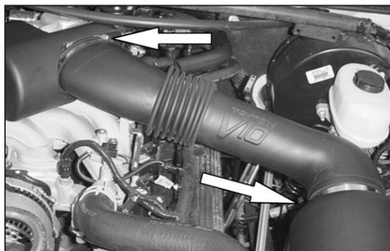
6. Loosen the hose clamps on the intake tube at the air cleaner and throttle body.
