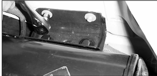
34. Tighten the two bolts that retain the evaporative canister mounting bracket to the inner fender.
