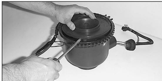
16. Using a flat blade screwdriver, push in and release the four clips that retain the mass air sensor retaining plate.
