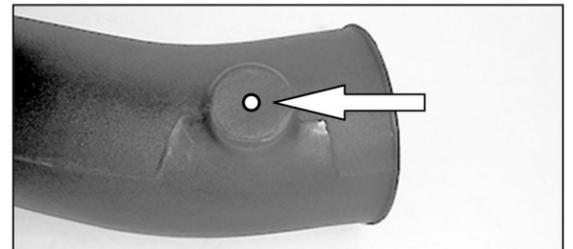
23. On models equipped with an external air temperature sensor, drill out the drill point in the K&N® intake tube using a 11/16" drill bit.
