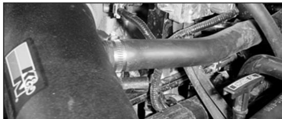
35. Attach the idle air control line to the large vent fitting on the intake tube
