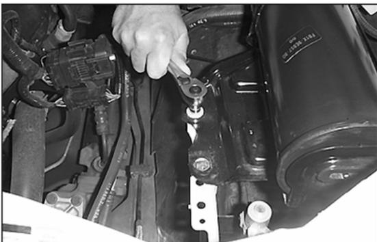
12. Loosen and remove the bolt that retains the evaporative canister mounting bracket.
