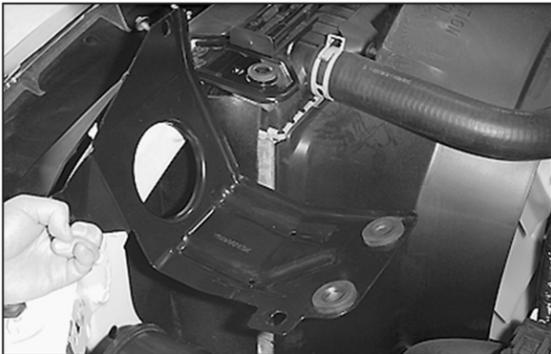
11. Remove the air cleaner mounting bracket.
