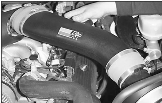
30. Install the intake tube.
