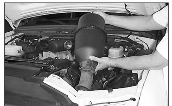
9. Pull upward firmly and remove the air cleaner.
