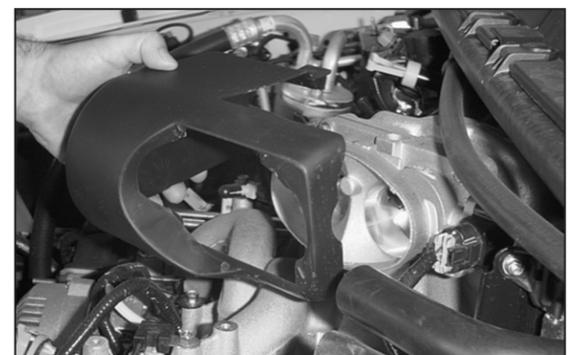
8. Remove the throttle body cover from the throttle body as it will not be reused.
