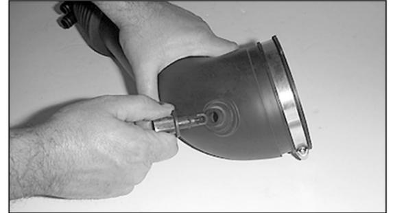
22. On models equipped with an external air temperature sensor, remove the air temperature sensor from the stock intake tube.
