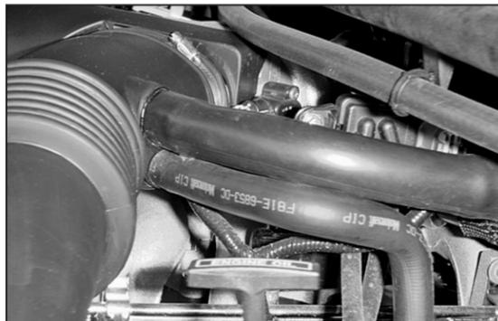
5. Detach the idle air control and PCV lines from the stock intake tube.
