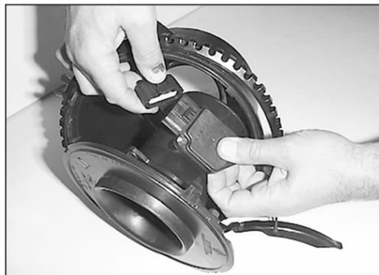
18. Disconnect the primary mass air sensor electrical connection.
