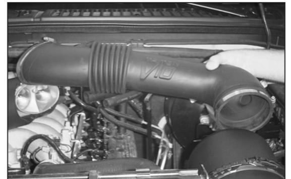
7. Remove the stock intake tube.
