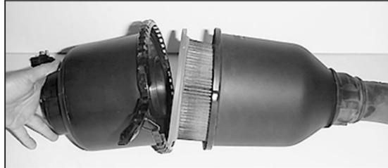
15. Disassemble the air cleaner assembly.
