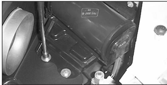
33. Position the heat shield for best alignment and tighten the hardware that retains it.
