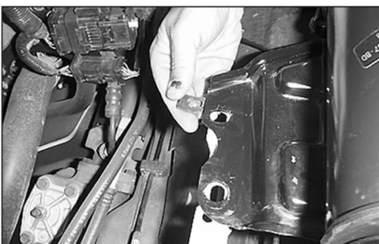
14. Remove the two clip nuts from the evaporative canister bracket lower mounting point.
