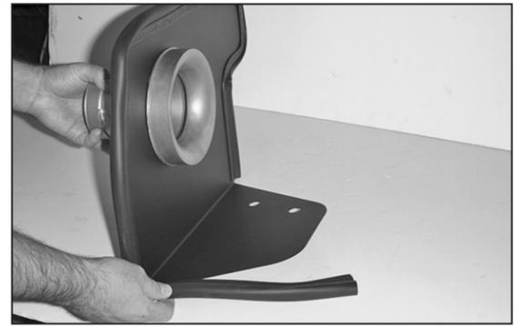
21. Install the trim seal onto the heat shield as shown.
