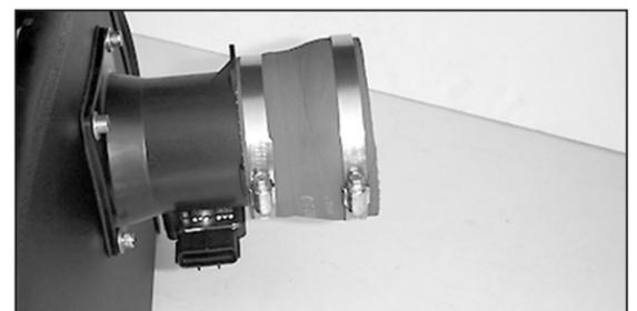
27. Install the stepped hose onto the flange of the mass air sensor and tighten hose clamp.
