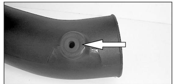
24. On models equipped with an external air temperature sensor, insert the grommet into the hole drilled in the K&N® intake tube.
