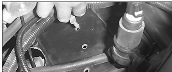
39. Reconnect the secondary mass air sensor electrical connection and reattach the wiring harness retaining clip to the inner fender apron.
