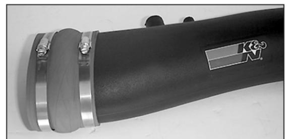
26. Install the hump hose onto the intake tube and tighten the hose clamp.
