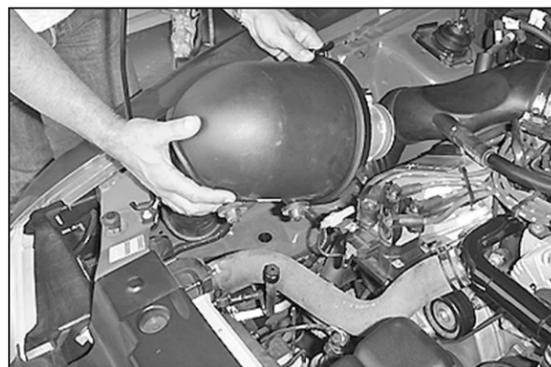
5. Pull the air cleaner assembly upward and remove from vehicle.
