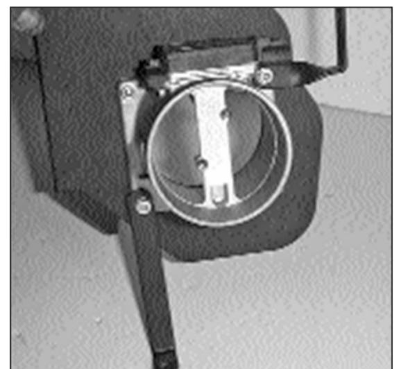
8. Assemble the mass air sensor, adapter, gaskets, heat shield and brackets using the hardware provided.
