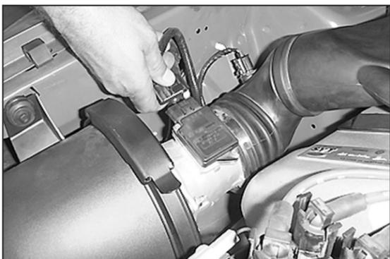
2. Disconnect the mass air sensor electrical connections.
