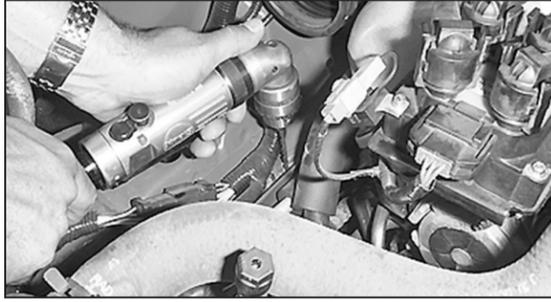
11. Remove the mass air assembly from the vehicle and using a 3/16" drill bit, drill out the two marks.
