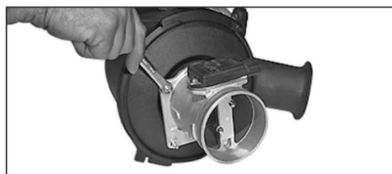
6. Loosen and remove the four nuts that retain the mass-air sensor to the air cleaner.
