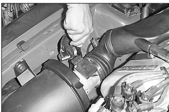
3. Loosen the hose clamp on the intake tube at the mass air sensor.
