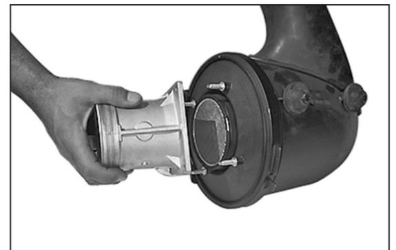
7. Remove the mass air sensor from the air cleaner.
