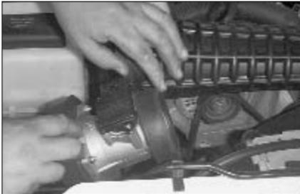
15. Install rubber intake adapter onto mass air sensor.
