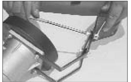
13. Using the hardware and support brackets provided, attach the mass air assembly to the airbox support bracket.
