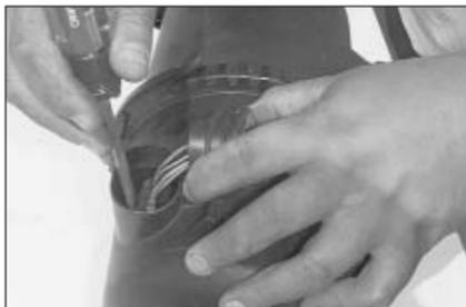
7. Pull rubber boot back away from airbox. Depress tab with screwdriver as shown to release electrical connection.
