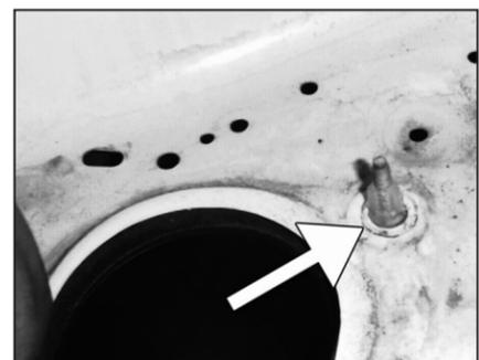
7. Using a pair of dykes, cut the three plastic clips from the air box mounting studs.
