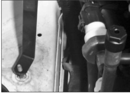
16. Place the "Z" bracket onto the original rear air box mounting stud and secure it with the provided hardware.
