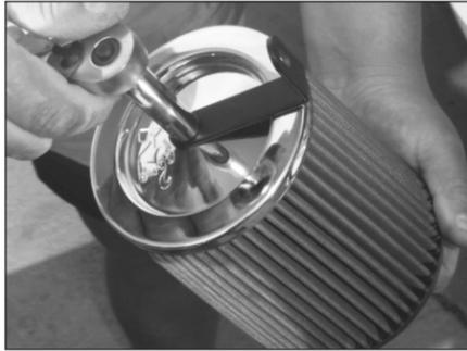
17. Attach the "L" bracket to the stud located on the top plate of the air filter element, secure with the provided nut.
