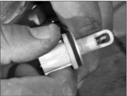
14. Insert the air temperature sensor into the slotted hole on the air temperature sensor bracket and turn 90 degrees to secure.
