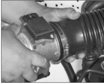
15. Insert the mass air assembly into the intake tube and secure with original hose clamp.
