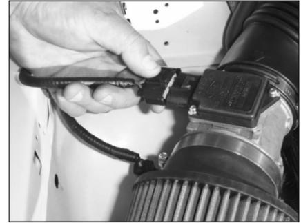
21. Reconnect the mass air sensor and the air temperature sensor electrical connections.
