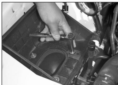
5. Using a 7/16" socket, loosen and remove the three nuts that secure the air box base.
