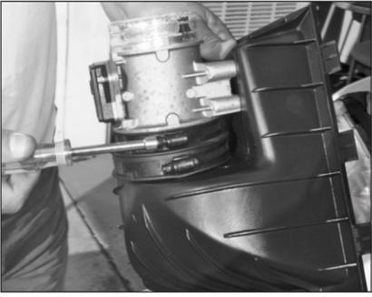
10. Remove the mass air sensor from the air box lid.
