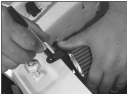
19. Line up the "L" bracket with the radiator core support. Position everything for best fit and clearance. Mark the "L" bracket hole, then remove the air filter and drill.
