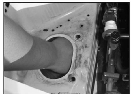
8. Once you have cut the clips from the mounting studs, push the scoop down into the cavity to remove the three threaded clips from the studs.
