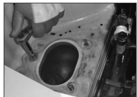
9. Assemble the provided hardware onto the two front mounting studs.
