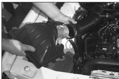
4. Release the over center clips on the air box and remove the air box lid from the vehicle.
