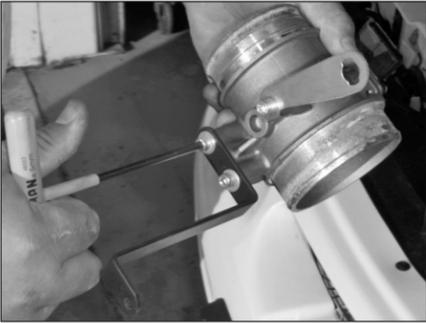
12. Attach the "Z" bracket and temperature sensor bracket onto the mass air sensor, secure with the provided hardware as shown.
