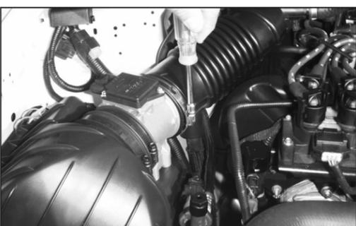
3. Loosen the hose clamp and remove the intake tube at the mass air sensor.
