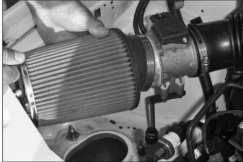
18. Install the air filter element onto the mass air sensor as shown.
