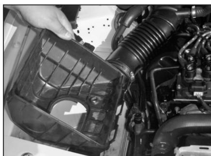
6. Remove the air box base as shown.
