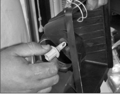
11. Remove the air temperature sensor from the air box lid.
