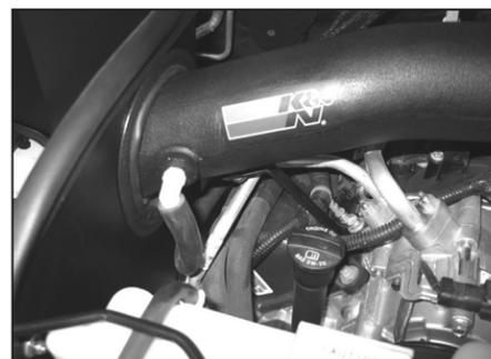
29. Connect the provided silicone vent hose to the modified factory vent tube and then connect the open end to the intake tube as shown.
