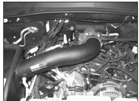
27. Install the intake tube into the silicone hose at the throttle body and align with the tube mounting bracket installed during step #11. Secure the intake tube with the provided hose clamp and hardware.
