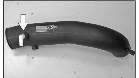
26. Install the 90° 1/4" npt fitting into the intake tube as shown.
