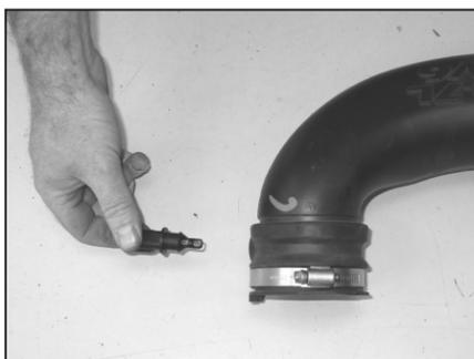
23. Remove the air temperature sensor from the factory intake tube as shown.
