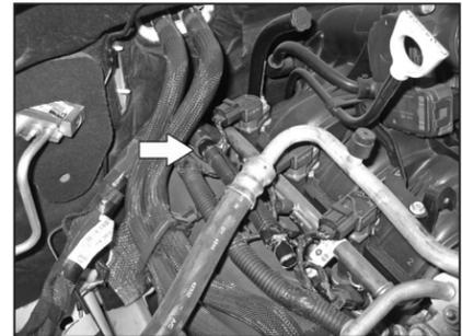
8. Reinstall the modified crank case vent tube onto the valve cover as shown.
