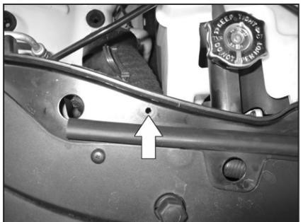
20. Drill a 1/4" O.D. hole at the marked location.
