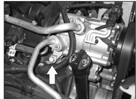
10. Remove the lower rear A/C compressor mounting bolt shown.
