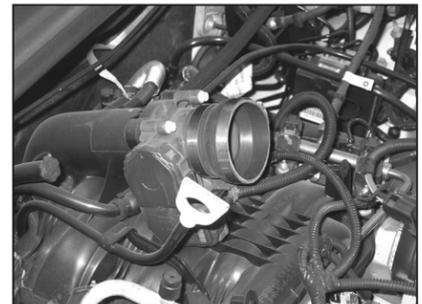
9. Install the silicone hose (084034) onto the throttle body and secure with the provided hose clamp.
