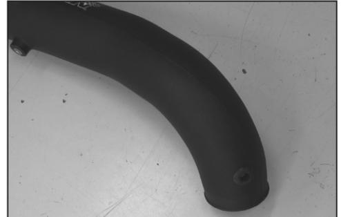
24. Install the supplied grommet into the intake tube as shown.
