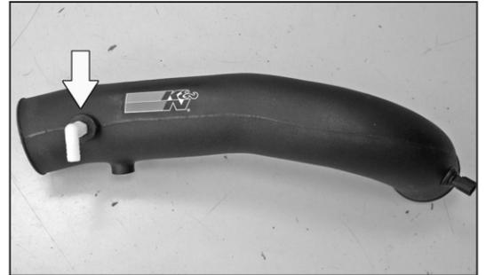
26. Install the 90° 1/4" npt fitting into the intake tube as shown.
