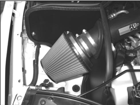
32. Install the filter assembly onto the intake tube and secure with the provided hose clamp.
