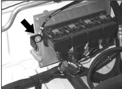
18. Install the heat shield mounting bracket (070066) onto the ECU and secure with the factory bolt removed in the previous step.
