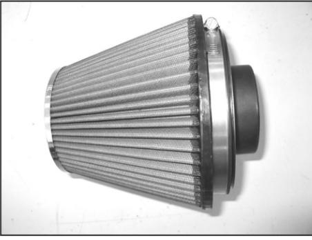
30. Install the filter adapter into the K&N air filter and secure with the provided hose clamp.
