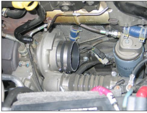
16. Install the provided silicone hose (08761) onto the turbo and secure with the provided hose clamp.
