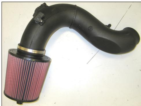
32. Install the K&N<sup>®</sup> Air Filter onto the intake tube and secure with the provided hose clamp.
