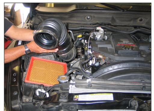
8. Remove the stock intake tube from the vehicle.
