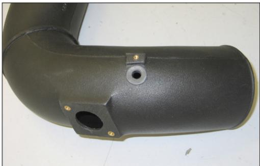
27. Install the provided grommet into the intake tube as shown.
