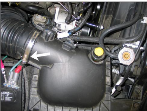
4. Loosen the hose clamp which secures the stock intake tube to the upper air box housing.
