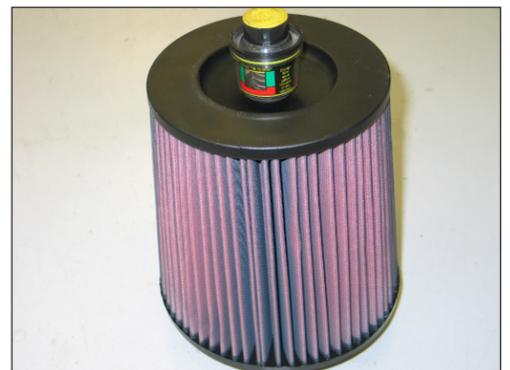
25. Install the grommet and filter minder removed in step 24 into the K&N® air filter as shown. On vehicles not equipped with filter minder install the provided plug.
