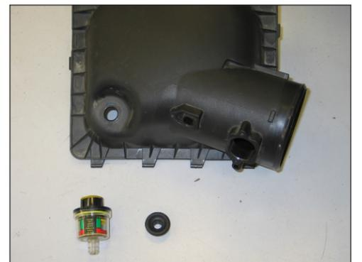
24. On vehicles equipped with filter minder, remove filter minder and grommet from the upper air box as shown.
