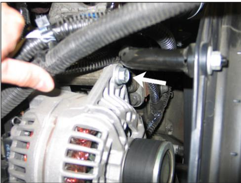
13. Remove the upper alternator mounting bolt shown.
