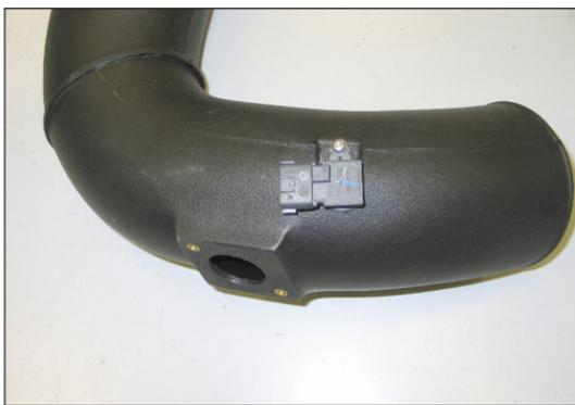
28. Install the air temperature sensor into the grommet and then secure the sensor with the provided bolt and spacer.
