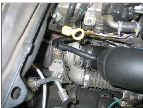
34. Install the provided air injection hose onto the air injection tube and then connect the open end to the 1/4" npt fitting in the K&N<sup>®</sup> intake tube.
