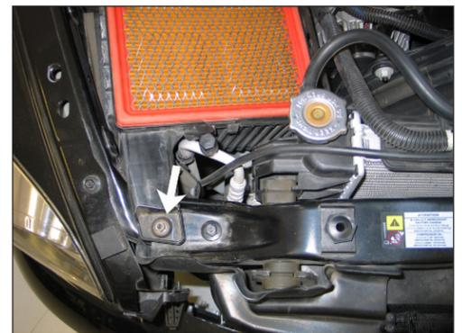
9. Remove the nut which secures the front of the lower air box housing to the radiator core support.
