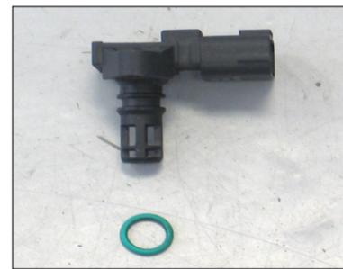
23. Remove the "O" ring from the air temperature sensor.
