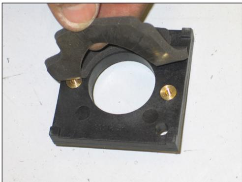
29. Apply the provided gasket onto the mass air sensor adapter as shown.
