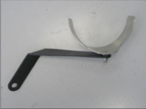
12. Install the supplied saddle clamp onto the tube mounting bracket (07160) using the provided hardware as shown.
