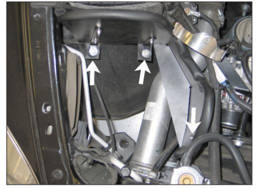
21. Install the heat shield assembly into the engine compartment as shown. The inserted nuts should be positioned into the air box mounting grommet holes and align the front mounting hole in the heat shield with bracket installed in step #15. Secure the heat shield with the provided hardware and the two inserted nuts.
