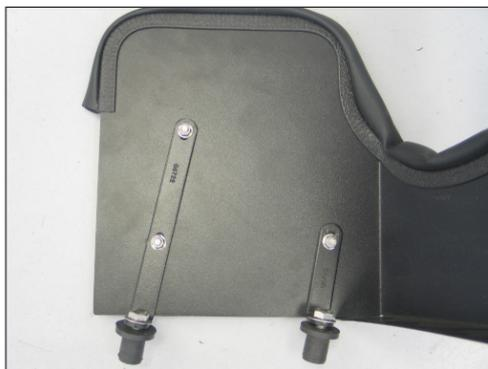
20. Attach the two provided inserted nuts to the heat shield using the provided hardware as shown.
