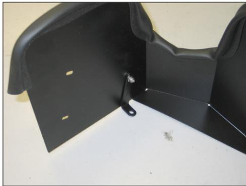
18. Install the heat shield mounting bracket (06723) onto the heat shield using the provided hardware.
