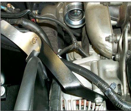
14. Install the tube mounting bracket assembly onto the alternator and secure with the factory bolt removed in the previous step.
