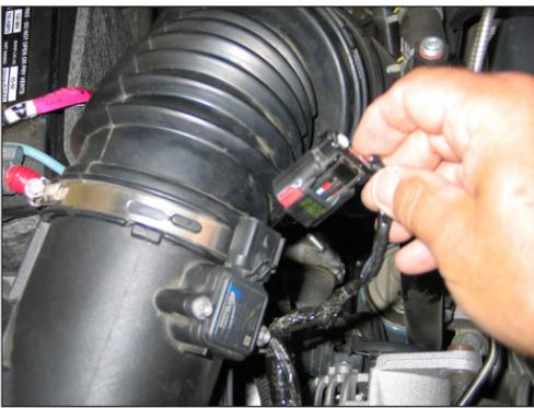
2. Release the red locking clip and then disconnect the mass air sensor electrical connection.
