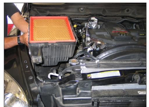
10. Firmly pull the lower air box assembly up to disengage it from the mounting grommets and then remove it from the vehicle.
