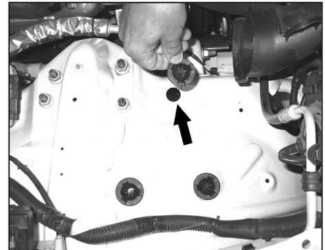
6. Remove the inner air box retaining grommet as shown.
