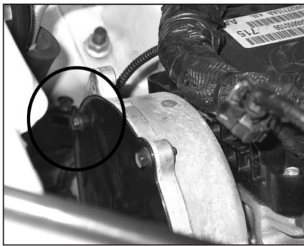
8. Remove the timing cover bolt (shown).
