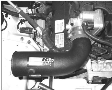
15. Install the K&N® intake tube into the silicone hose at the throttle body and align the mounting bracket with the timing cover bolt location (removed in step #8).
