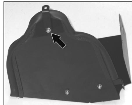
22. On 2007 model year vehicles, install the heat shield mounting bracket (#07805) to the side of the heat shield using the provided hardware.
