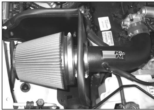
27. Install the K&N® filter assembly onto the intake tube and secure with the provided hose clamp. Then connect the crank case vent line to the hose mender as shown and secure with the provided hose clamp.
