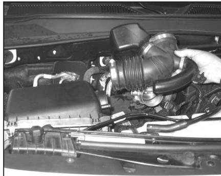
4. Loosen the two hose clamps that secure the stock intake tube, then remove the stock intake tube as shown.
