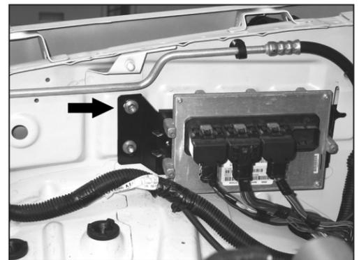
7. On 2007 model year vehicles, remove the ECU mounting nut shown.
