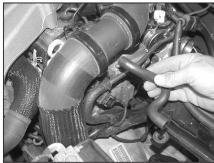
6. Disconnect the crankcase vent line from the valve cover as shown.
