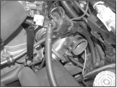
12. Install the provided silicone hose (08405) onto the turbo inlet as shown with the provided hose clamp.
