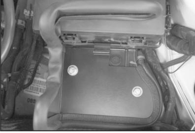
11. Install the heat shield onto the vehicle with the provided hardware as shown.
