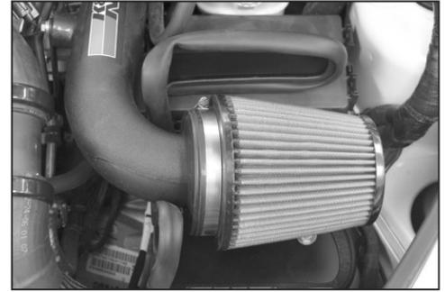
19. Install the air filter onto the intake tube as shown.
