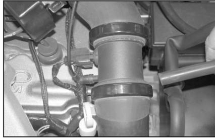
15. Connect the silicone hose with vent fitting on the valve cover as shown.
