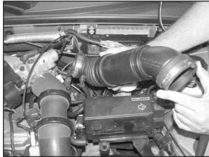
4. Loosen hose clamp at the turbo then remove the intake tube from the vehicle.
