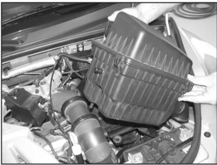
3. Lift firmly up on the airbox to remove from vehicle, then disconnect the crankcase vent from the airbox.
