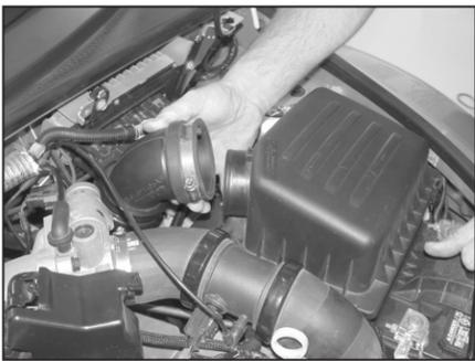
2. Loosen hose clamp at the airbox, then remove intake tube from the airbox as shown.
