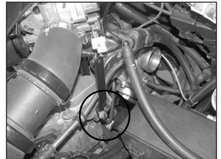
8. Install the new bracket onto the cylinder head with the provided hardware.
