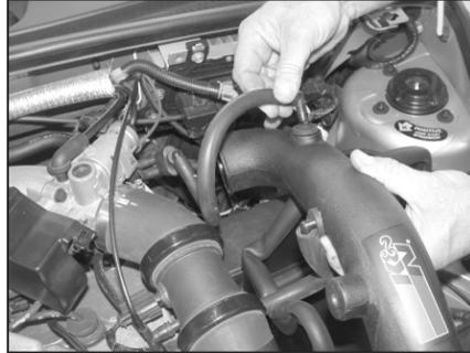
16. Reconnect the two vent fittings onto the new intake tube as shown.
