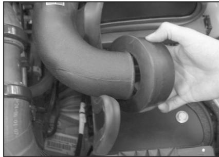
18. Install the air filter adaptor onto the intake tube as shown.
