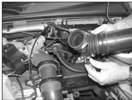
5. Disconnect the vacuum line from the intake tube as shown.
