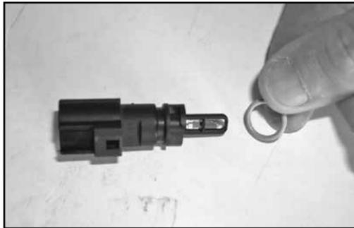
18. Remove the O-ring from the air temp. sensor as shown.
