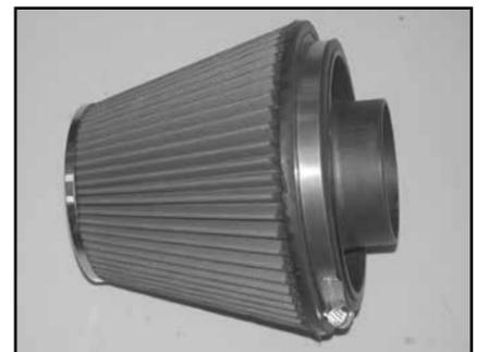
26. Install the filter adapter into the air filter as shown and secure with the provided hose clamp.
