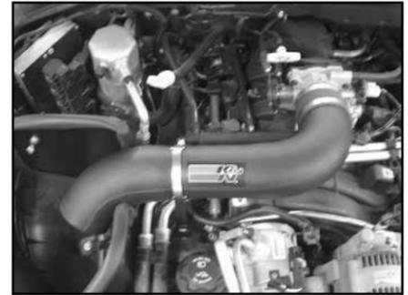
23. Install the K&N® intake tube into the silicone hose at the throttle body and onto the saddle clamp, then secure with the provided hose clamps.
