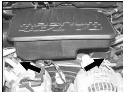
5. Loosen and remove the two intake plenum mounting bolts indicated
