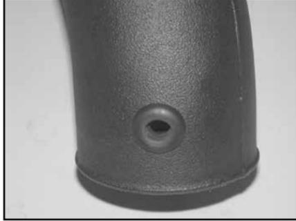
17. Install the provided grommet into the K&N® intake tube as shown.
