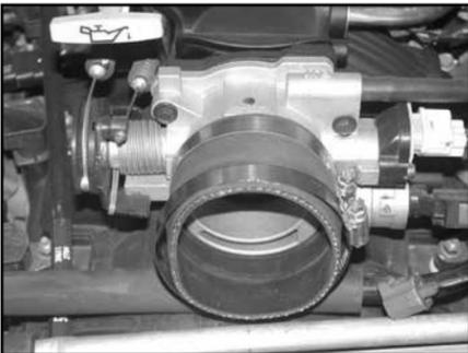
15. Install the silicone hose (08051) onto the throttle body and secure with the provided hose clamp as shown.
