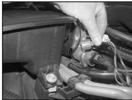
4. Depress the locking tab on the air temperature sensor electrical connection and then pull to disconnect the sensor electrical connection.
