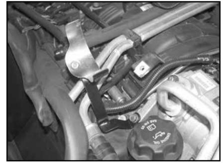
22. Using the bolt removed in step #21, install the tube mounting bracket onto the A/C compressor as shown.
