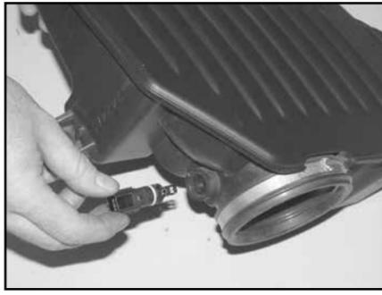
16. Twist the air temperature sensor counter clockwise and remove it from the stock intake plenum.
