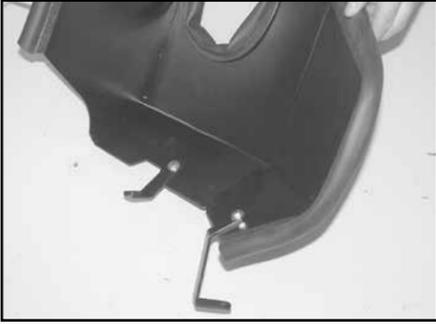
11. Install the "C" bracket (010123) onto the heat shield with the provided hardware as shown.
