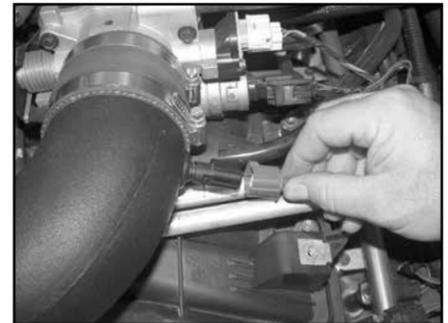
24. Reconnect the air temperature sensor electrical connection as shown.
