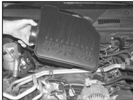
6. Lift and remove the intake plenum from the vehicle as shown.
