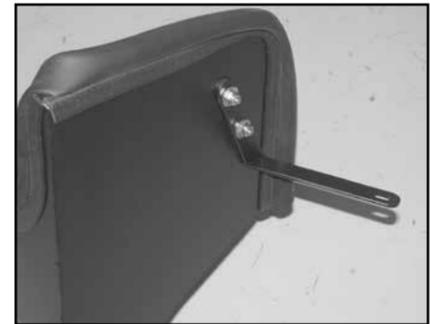
9. Install the "L" bracket (010124) onto the heat shield with the provided hardware as shown.
