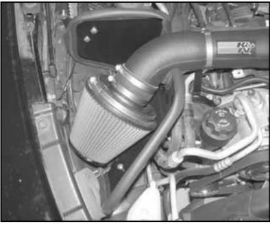
28. Install the air filter assembly onto the K&N® intake tube and secure with the provided hose clamp as shown.
