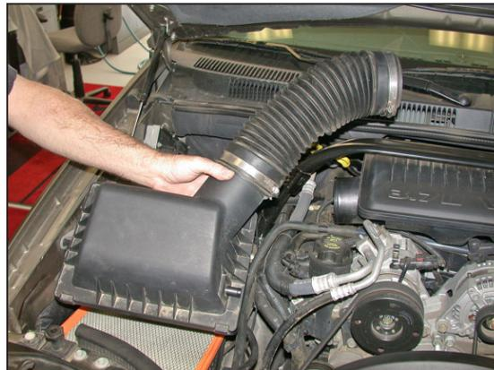
3. Unclip the upper airbox retaining clips and remove the upper airbox and intake tube assembly as shown.
