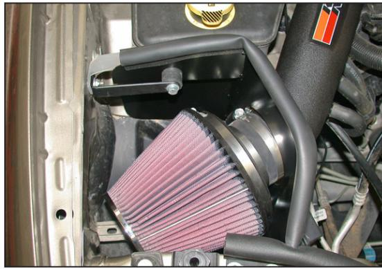
29. Install the air filter assembly onto the K&N® intake tube as shown and secure with the provided hose clamp.
