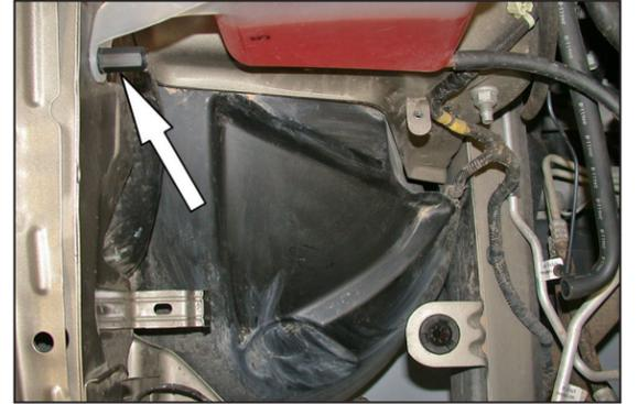
19. Remove the coolant reservoir-retaining nut and airbox mounting grommet shown.
