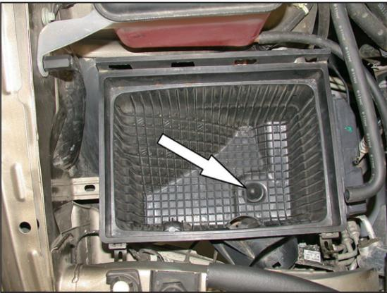
8. Remove the airbox mounting bolt shown.
