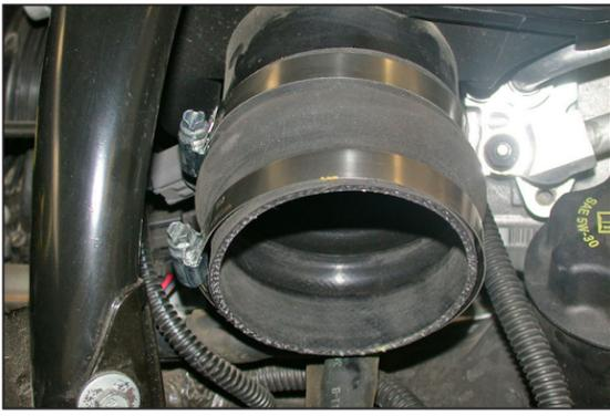
24. Install the silicone hose (08699) onto the intake plenum and secure with the provided hose clamp as shown.
