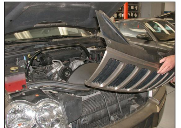
6. Remove the six grill retaining clips from the grill, then tilt the grill forward and lift to remove from the vehicle.
