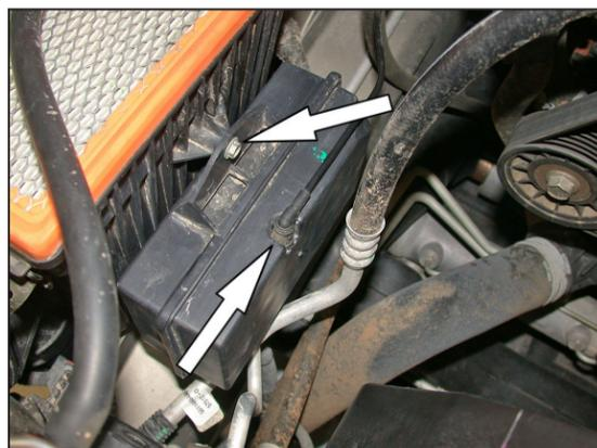
4. Disconnect the vacuum canister hose shown.
