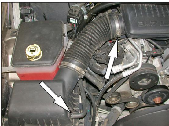
2. Loosen the hose clamp, which secures the stock intake tube to the intake plenum, and disconnect the crankcase vent hose from the airbox lid.
