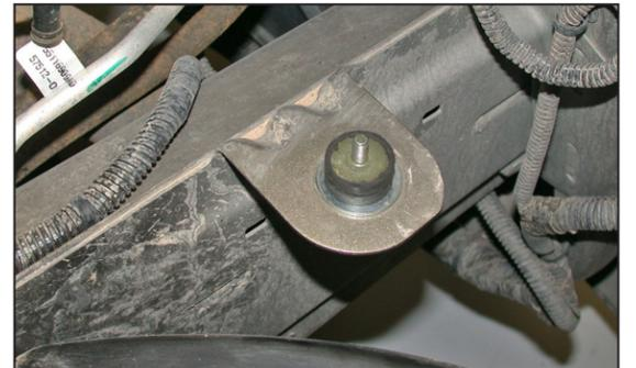
20. Using the two fender washers and one rubber washer, install the 6mm male/female rubber mounted stud onto the lower airbox mount as shown.
