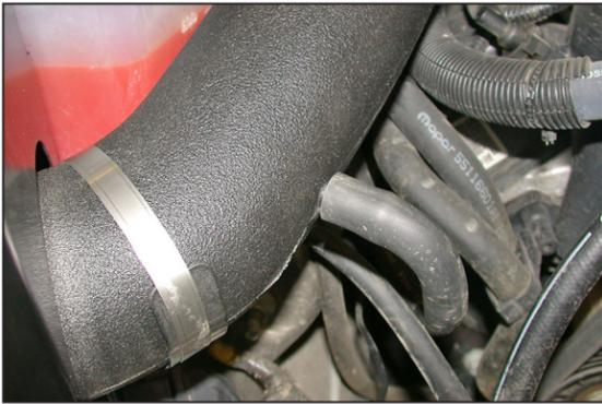
26. Connect the crankcase vent hose onto the K&N® intake tube as shown.
