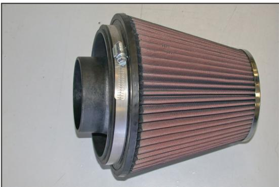
27. Install the filter adapter into the air filter as shown, secure with the provided hose clamp.
