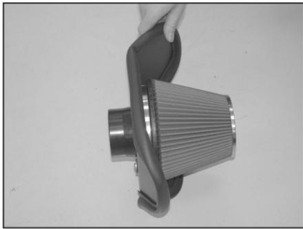
11. Install the K&N® air filter onto the filter adapter as shown.
