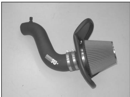
18. Install the air filter assembly onto the K&N® intake tube as shown.
