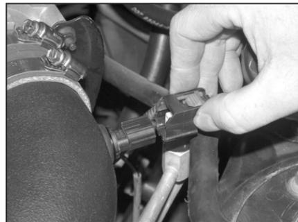
22. Reconnect the air temperature electrical connection as shown.
