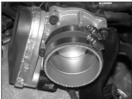
19. Install the silicone hose (08190) onto the throttle body and secure with the provided hose clamp as shown.
