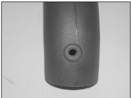
14. Install the provided grommet into the small throttle body end of the intake tube.
