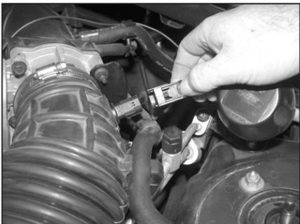
2. Unlock the red locking tab on the air temperature sensor electrical connection, then depress the locking lever and pull apart the temperature sensor electrical connection
