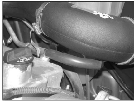
21. Install the provided silicone vent hose onto the valve cover vent and onto the elbow into the K&N intake tube as shown.
