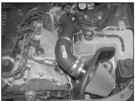
20. Install the K&N® intake assembly into the silicone hose at the throttle body and onto the saddle clamp as shown, then secure with the provided hose clamps. Adjust the air filter assembly for best clearance and tighten the hose clamp, which secures it to the K&N® intake tube.
