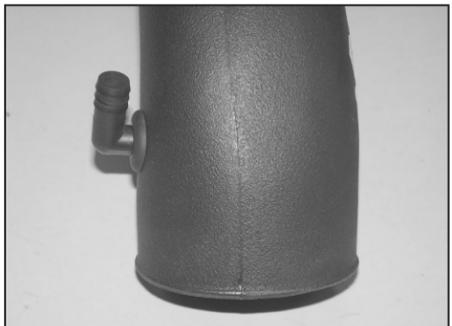
17. Install the provided elbow fitting into the grommet installed in step #16 as shown.
