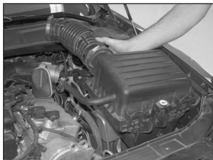
6. Lift the complete intake and air filter assembly to remove it from the vehicle.
