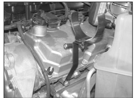
8. Using the provided hardware, install the tube-mounting bracket onto the engine at the threaded hole in the cylinder head as shown.
