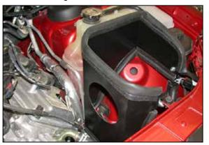
11. Install the heat shield assembly into the vehicle and secure to the bracket installed in step #8. Then secure the "L" bracket with the factory bolt removed in step #6 to the air box mounting location.
