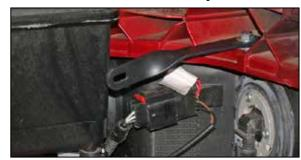
8. Install the twist bracket (070772) onto the core support using the hardware provided through the existing hole as shown.
