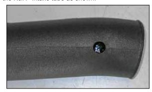
16b. Drill out the hole in the intake tube to 0.75".
