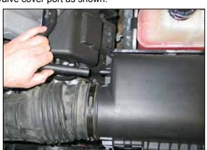
5a. On SRT-8; 6.1L vehicles, disconnect the crank case vent hose from the air box as shown.
