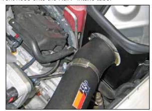
19a. On SRT 8; 6.1L equipped vehicles, connect the factory crank case vent hose onto the 90° fitting installed into the K&N® intake tube (in step #16c).
