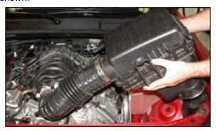
7. Lift the complete intake and air filter assembly to remove it from the vehicle.
