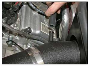
19. Install the provided crank case vent hose onto the vent port on the valve cover then install the vent hose onto the K&N® intake tube.
