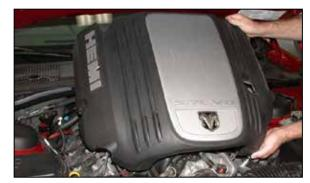
2. Lift up on the engine cover to loosen it from the mounts, and then remove the cover from the vehicle.
