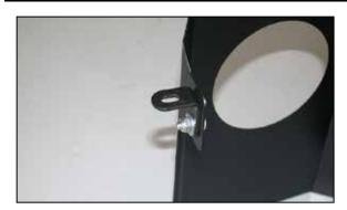
9. Install the "L" bracket (070066) onto the heat shield with the provided hardware through the non-slotted hole in the bracket.
