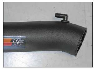
16d. On SRT 8; 6.1L equipped vehicles, install the provided 90° hose mender as shown.
