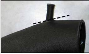
16a. On SRT 8; 6.1L vehicles, cut the vent off of the  $K\&N^{\odot}$  intake tube as shown.
