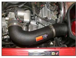
18. Install the K&N® intake tube into the throttle body and onto the saddle clamp as shown, then secure with the hose clamps provided.
