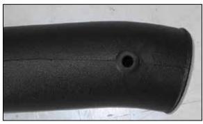
16c. On SRT 8; 6.1L equipped vehicles, install the provided grommet into the 0.75" ID hole as shown.
