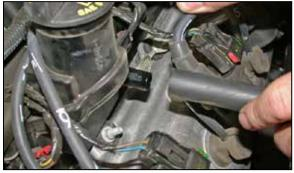
5. Disconnect the crank case vent hose from the valve cover port as shown.
