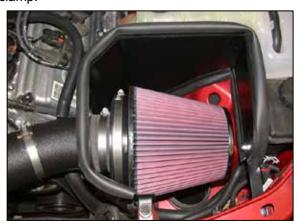
22. Install the air filter assembly onto the K&N<sup>®</sup> intake tube and secure with the provided hose clamp as shown.
