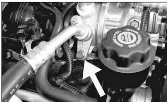
17. Remove the A/C compressor-mounting bolt.
