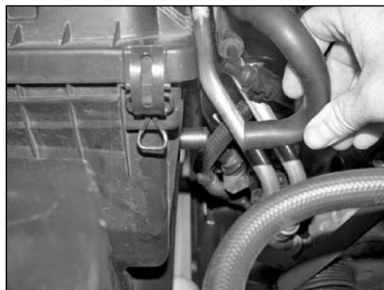
4. Disconnect the stock crankcase vent hose from the airbox as shown.
