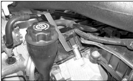
24. On vehicles not equipped with A/C, use the spacer and bolt provided to secure the mounting bracket to the engine.
