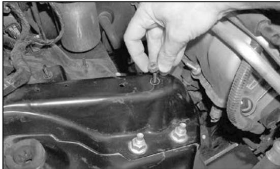
15. Vehicles that do not come equipped with cruise control, install the provided spacer and washer onto the stud as shown.
