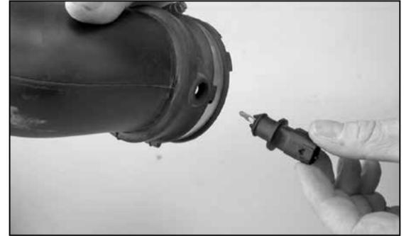
20. Remove the air temperature sensor from the stock intake tube as shown.
