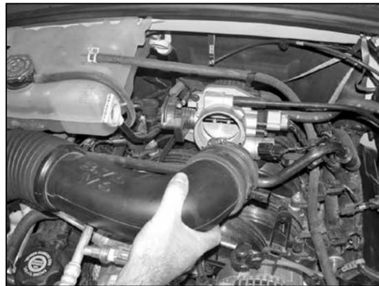
3. Loosen the hose clamp that secures the intake tube to the throttle body, and then disconnect the intake tube from the throttle body.
