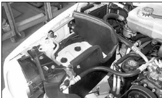
16. Install heat shield onto the vehicle with the provided hardware as shown.
