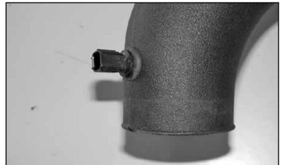
21. Install the air temperature sensor into the grommet in the K&N® intake tube as shown.
