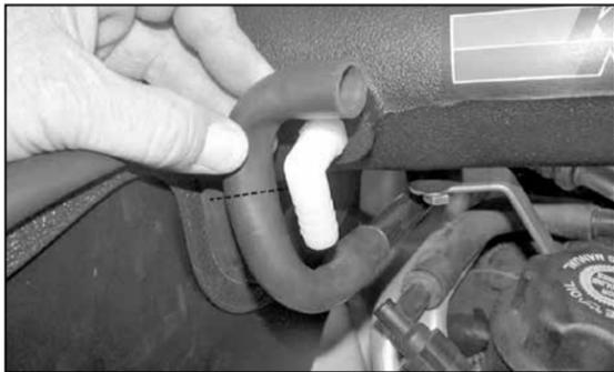
25. Rotate crankcase vent hose, align with NPT fitting, and cut where shown.
