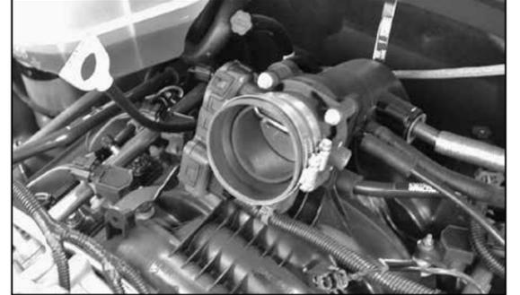
18a. On 2007 vehicles with a plastic throttle body, install the supplied silicone hose (084034) onto the throttle body and secure with the provided hose clamps as shown.
