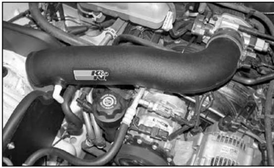
23. Install the K&N® intake tube into the silicone hose at throttle body, position the tube mounting bracket to line up on the A/C pump with the bolt removed in step #17. Then secure bracket to intake tube with the provided hardware. Then tighten the hose clamp at the throttle body and the AC mounting bolt removed in step #17.
