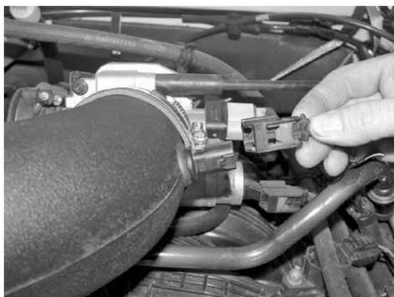
27. Reconnect the air temperature sensor electrical connection as shown.
