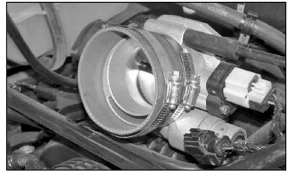
18. On 2006 and earlier vehicles, install the provided silicone hose (08690) onto the throttle body with the provided hose clamps as shown.
