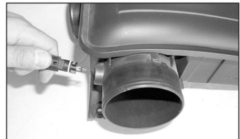
25. On models that come equipped with temp sensors, remove the air temp sensor from the resonator box as shown.
