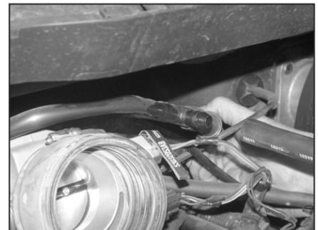
8. On 2007 and earlier model vehicles, remove crankcase vent hose from tee as shown.
