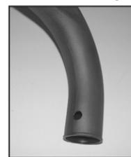
25b. On models that come equipped with temp sensors, drill a 7/8" hole in the K&N® intake tube at the drill point.
