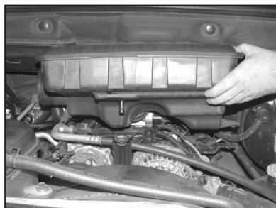
6. Pull up firmly to release the resonator from the engine.
