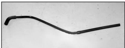
29A. On 2008 and later model year vehicles remove the crankcase vent tube from the passenger side valve cover. Then remove the rubber elbow from the tube, and install the provided straight silicone hose. Then reinstall the crankcase vent tube so that it runs behind the throttle body .
