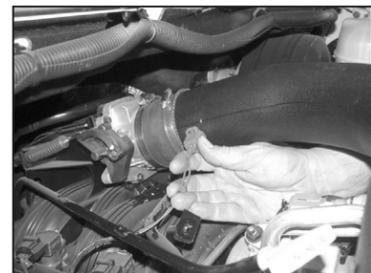
25a. On vehicles equipped with an air temperature sensor, hold up the air temperature sensor wiring harness to the intake tube and mark the intake tube for drill point.
