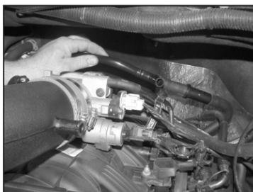
34. Reinstall the vent tube assembly into the rubber fittings in each valve cover so that the "T" fitting is now on the drivers side of the engine facing forward.
