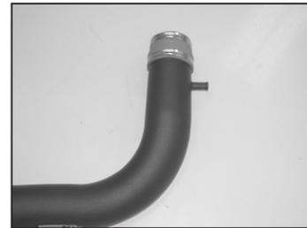
23. Install the provided silicone hose (08051) onto the K&N® intake tube with the provided hose clamp as shown.
