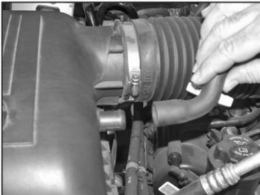
2a. On vehicles equipped, disconnect the crankcase vent from the airbox as shown.
