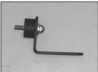
16A. On 2008 and later model year vehicles: Install the provided rubber mounted stud onto the heat shield mounting bracket (26607) as shown.
