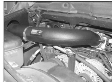
24. Install the intake tube onto the throttle body and saddle clamp and secure with the provided hose clamps as shown.
