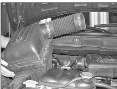
3. Lift firmly to release the airbox from the mounting studs, then remove completely.
