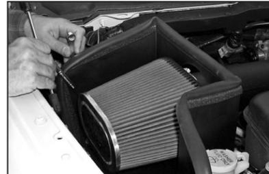
37. Align the heat shield for best clearance then tighten all the brackets.
