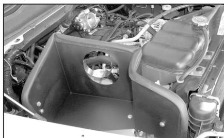
22. Install the heat shield onto the factory airbox studs then mount to the previously installed brackets.
