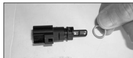
25d. Remove the O-ring from the air temp. sensor as shown.
