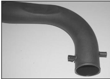
25e. Install the air temp sensor into the K&N® intake tube as shown.
