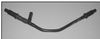
33. Rotate the long side of the vent tube assembly 180° as shown.
