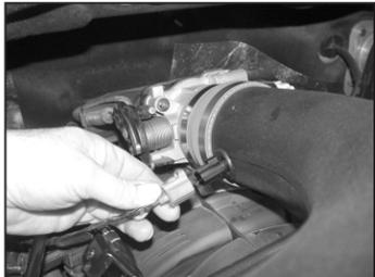
28. On models equipped with a air temp sensor, reconnect the electrical connection as shown.
