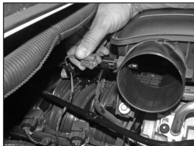
4. On vehicles equipped with a air temperature sensor in the resonator box, depress the locking tab and separate the electrical connection.
