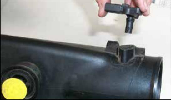
11. Remove the temperature sensor from the air box lid using an 9/32 socket.
