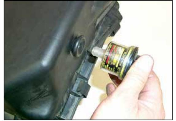
21. Remove the air filter minder and grommet from the stock air box lid as shown.
