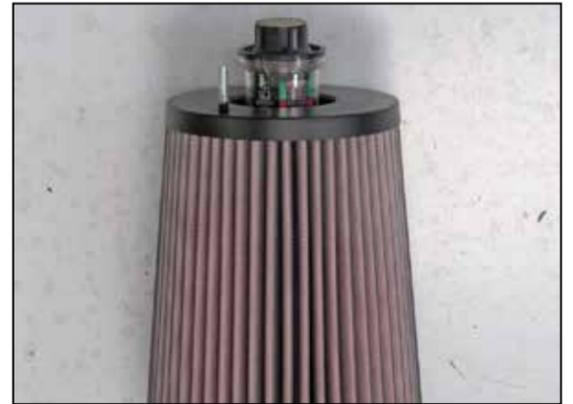
23. Install the grommet and air filter minder that was removed in step 21 onto the K&N® air filter as shown.
