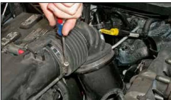
3. Loosen the hose clamps at the turbo inlet and the air box outlet as shown.
