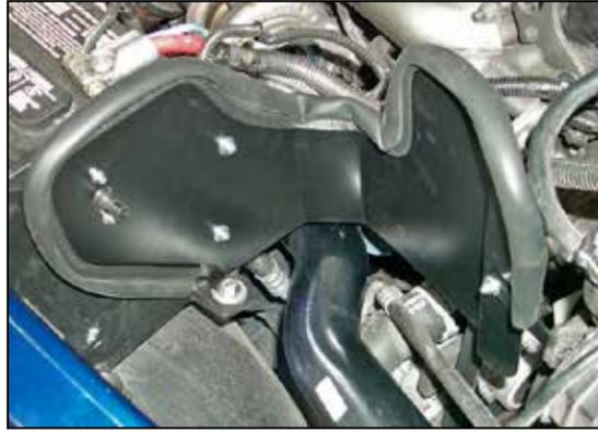
16. Install the heat shield onto the vehicle with the provided hardware.
