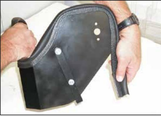
10. Install the edge trim onto the heat shield as shown.
