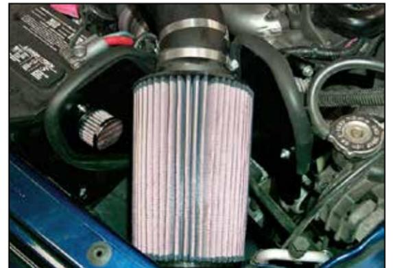
25. Install the K&N® air filter onto the intake tube as shown.
