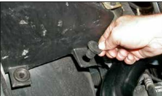
14. Install the nut insert onto the air box mounting tab as shown.
