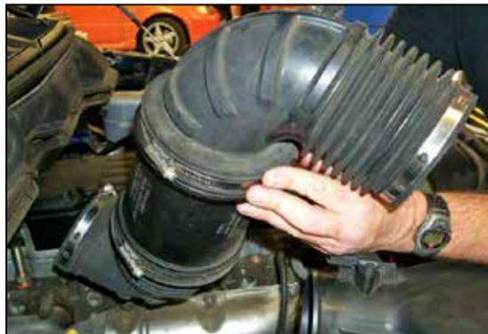
4. Remove the intake tube from the vehicle as shown.
