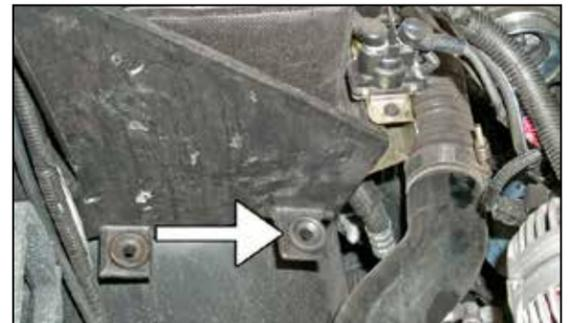
7. Remove the air box mounting grommet as shown.
