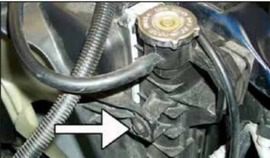
13. Remove the bolt that retains the fan shroud to the radiator.
