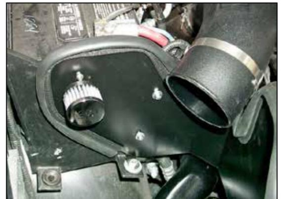
24. Install the K&N® air filter onto the air temperature sensor as shown.
