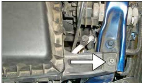
5. Loosen and remove the 10mm nut that retains the air box to the vehicle.
