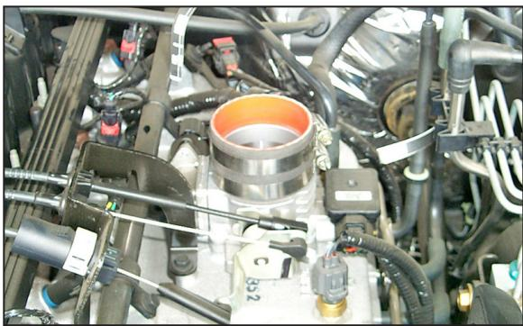
10. Install the provided silicone hose and hose clamps onto the throttle body as shown.
