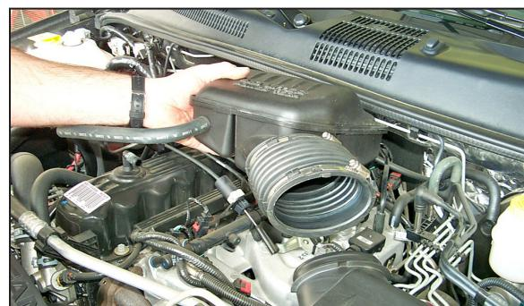
4. Loosen the hose clamp at the air cleaner lid and at the throttle body, then, remove the resonator and bellows assembly as shown.
