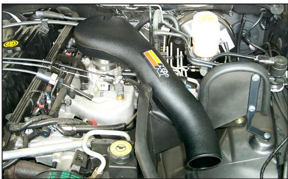
11. Install the K&N® intake tube into the silicone hose as shown, but do not tighten completely as some adjustment may be necessary.
