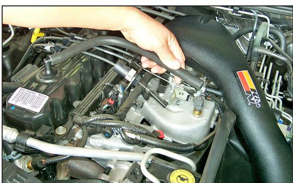
12. Connect the provided hose to the vent on the valve cover, then, connect the other end to the vent on the K&N® intake tube as shown.
