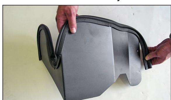
6. Install the provided trim seal onto the heat shield as shown. Trim if needed.
