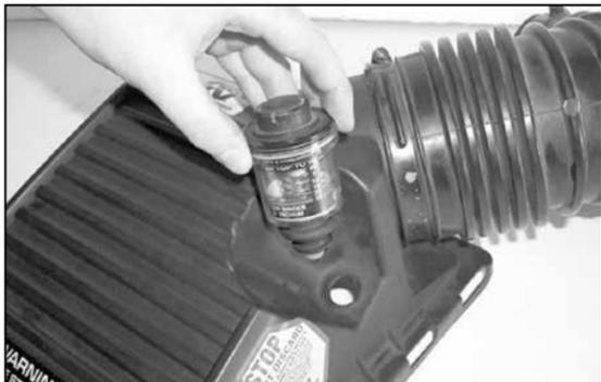
13. Remove the filter restriction gauge and grommet from the stock airbox as shown.
