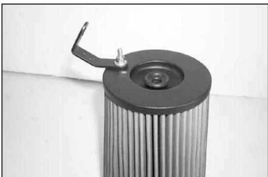
12. Install filter bracket provided onto the stud on the top plate of the air filter as shown.
