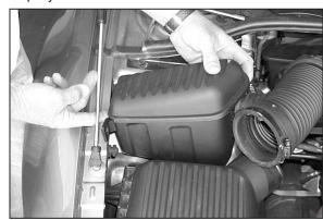
5. Loosen Hose Clamps, and remove Center Intake Tract and Hose from Front Intake Assembly in an upward direction.
