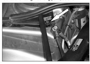
20. Install Bolt in existing Cowl Bolt Location and hand tighten, as shown.
