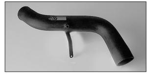
14. Clean the inside of the K&N<sup>®</sup> Intake Tube and attach the "L" Bracket using (2) 1/4-20x1/2"Long Bolts and (2) Wave Washers, supplied.
