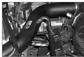
24. Replace Stock Vent Hose to engine and K&N $^{\! \rm B}$  Intake Tube.
