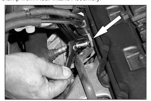
12. Loosen Bolt and remove Airbox Bracket. (Bolt will be reused.)
