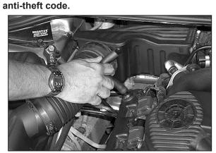
2. Remove the Vent Hose from the Airbox and Engine. (Vent Hose will be reused.)
