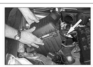
6. Lubricate Grommet and remove Airbox, as shown.
