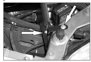
23. Tighten Heat Shield Bracket Bolts, as shown.
