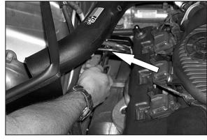
22. Center Intake Tube in the Heat Shield Hole and tighten bracket bolts under Intake Tube, as shown.
