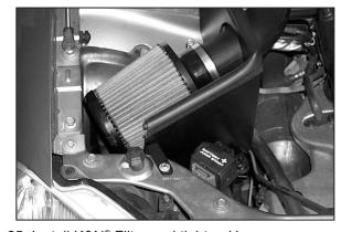
25. Install K&N® Filter and tighten Hose Clamp.
