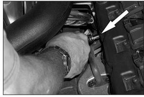
19. Using Stock Bracket Bolt, mount Intake Tube Bracket to existing mounting point, as shown.
