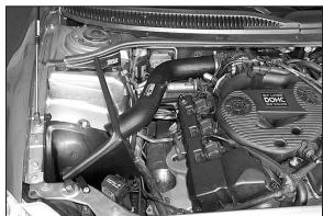
18. With Heat Shield in position, install K&N $^{\circ}$  Intake Tube, as shown.
