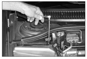
15. Remove Bolt from Cowl, behind Negative Battery Cable Location, using 13mm Socket.
