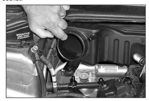
10. Lubricate Grommet and remove Rear Intake Assembly.
