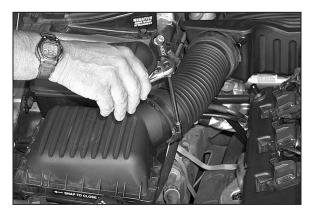
3. Loosen both Hose Clamps on Intake Hose.
