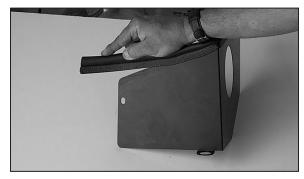
17. Install Edge Trim on the Heat Shield, as shown. Trim excess Edge Trim with Side Cutters, if necessary.
