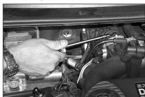
13. Place #56 Hose Clamp (supplied) on the Throttle Body Hose and reinstall it onto the throttle body. (Tighten Hose Clamp.)
