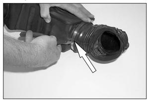
11. Using Side Cutters, cut and remove Band Clamp from Rear Intake Assembly.
