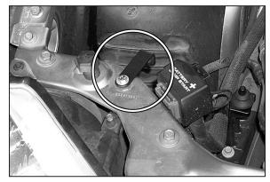
16. Attach Small "L" Bracket to the existing hole, located behind the Passenger Side Headlight, using a 6mm Bolt, 2 Washers, and a Nylock Nut. (DO NOT tighten completely. Adjustments will be made later.
