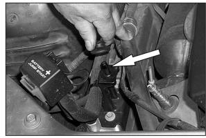
8. Place Grommet back onto existing Stock Airbox Bracket location.
