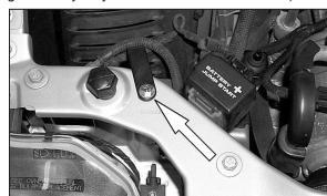
20. Install small Heat Shield Bracket on hole located behind the passenger-side headlight, using a 6mm Bolt, (2) Flat Washers, and a Lock Nut. (Hand tighten Only. Adjustments will be made later.)
