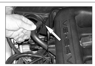
6. Remove Vent Hose from Rear Intake Tract Assembly. (DO NOT remove from engine.)
