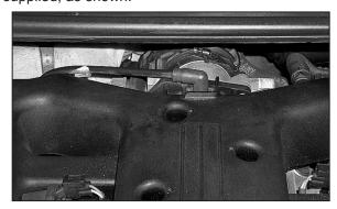
11. Reinstall Throttle Body Hose to throttle body and tighten Hose Clamp.
