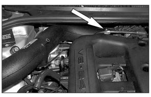
21. Install Intake Tube into Throttle Body Hose, as shown.
