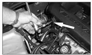
12. Using a 3/8" Drive Ratchet and a 13mm socket, remove stock Bolt, as shown. (Bolt will be reused.)
