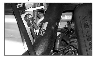
24. Hand tighten Cowl Bolt back into the stock location.
