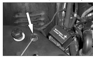
18. Using a Flathead Screwdriver, remove the stock plastic socket-head capscrew.
