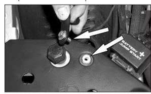
19. Place the white, nylon Spacer, as shown, and install the Heat Shield Bracket on hole located behind the passenger-side headlight, using a 6mm Bolt, (2) Flat Washers, and a Lock Nut.. (Hand tighten Only. Adjustments will be made later.)
