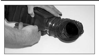
9. Remove Metal Band by cutting with Sidecutters.
