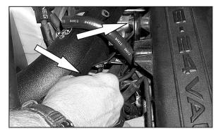
25. Tighten all bolts on brackets, as shown.
