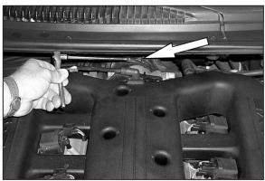
7. Loosen Hose Clamp at the Throttle Body using a 1/4" socket.
