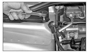
14. Remove Cowl Bolt located above the Negative Battery Cable, using a 3/8" Drive Ratchet and a 13mm socket. (Bolt will be reused.)
