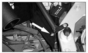
23. Attach Heat Shield to Bracket, using a Bolt, Washer and Nylock Nut provided.
