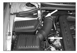
2. Loosen the Hose Clamps, using an 8mm socket.
