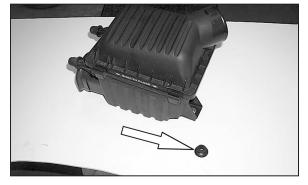
15. Remove Grommet from Airbox, as shown.
