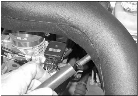
14. Connect the other end of the silicone hose to the vent on the K&N® intake tube
