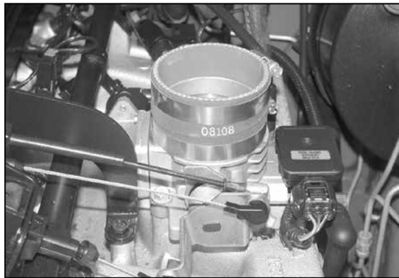
11. Install the silicone hose and hose clamps onto the throttle body as shown.
