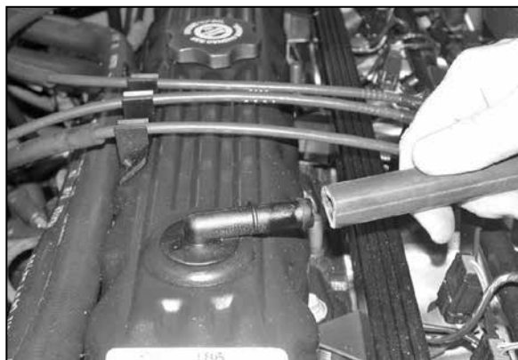
13. Install the provided silicone hose onto the vent on the valve cover.
