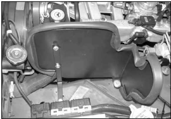
10. Using the provided hardware secure the “L” bracket to the inner fender as shown. Now tighten all hardware.
