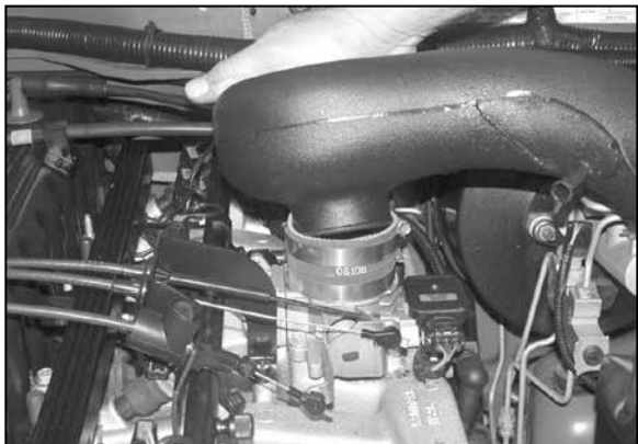
12. Install the K&N® intake tube into the silicone hose on the throttle body.
