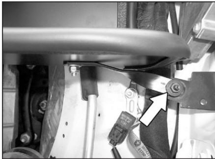
16. Using the nut that was removed in step 6, secure the bracket to the air box mounting stud as shown. Do not completely tighten at this time.
