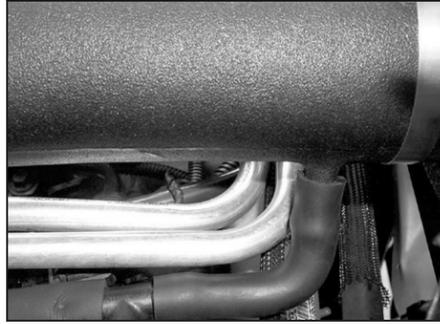
27. Connect the vent hose onto the K&N® intake tube as shown.
