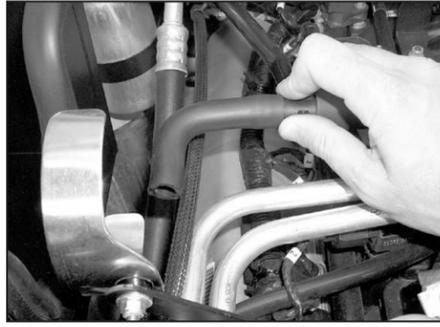
26. Re-install the vent hose onto the vent line as shown.
