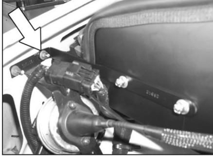
15. Using the nut that was removed in step 13, secure the bracket to the inner fender well.
