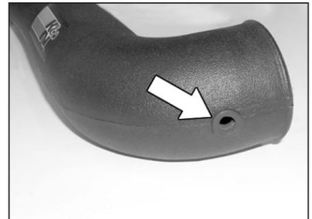
21b. Install the provided grommet into the intake tube as shown
