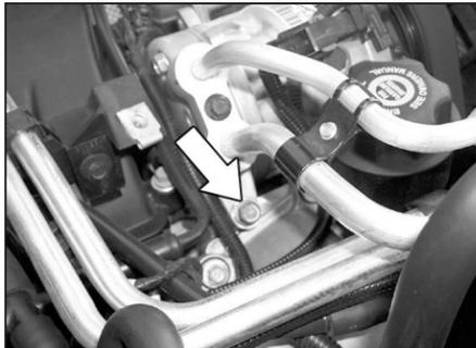
19. Remove the bolt from the A/C compressor as shown.
