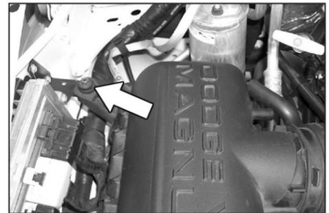
6. Loosen and remove the nut that retains the air box to the vehicle.
