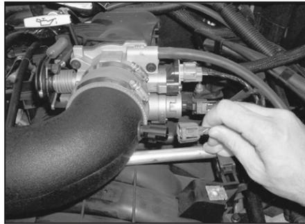
28. On vehicle's that come equipped with an air temperature sensor, re-connect the electrical connection as shown.
