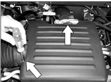
2. Loosen the hose clamp at the throttle body and air intake tube as shown.
