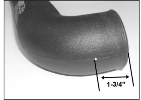
21a. On models that come equipped with an external temperature sensor, mark the intake tube 1-3/4" from the end of the tube, then drill a 3/4" hole into the intake tube.
