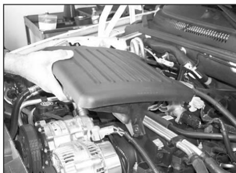
4. Remove the air resonator from vehicle as shown.
