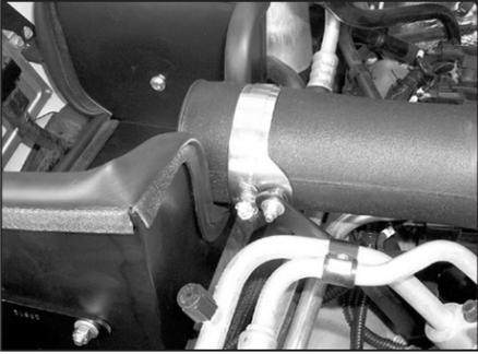
24. Secure the saddle bracket onto the K&N® intake tube with the provided hose clamp as shown.
