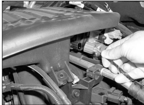
3a. On vehicles that come equipped with an air temperature sensor, disconnect the electrical connection as shown.
