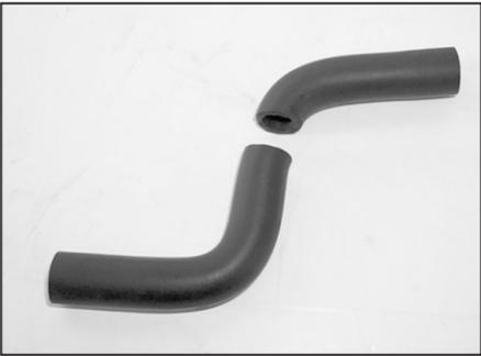
25. Cut the vent hose that was removed in step 23 as shown.
