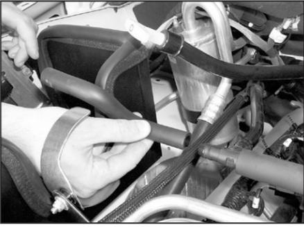
23. Remove the vent hose from the vehicle as shown.
