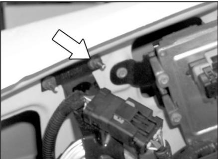
13. Remove the nut that retains the cruise control bracket to the inner fender.
