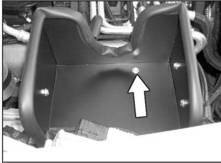
17. Attach the heat shield onto the lower "Z" bracket with the provided hardware.
