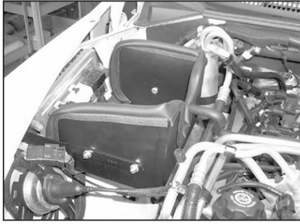
14. Install the heat shield into the vehicle as shown.
