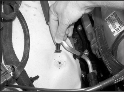
8. Unscrew the plastic air box retaining stud from the vehicle as shown.
