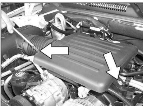
3. Loosen and remove the two bolts that retain the air resonator to the intake manifold as shown.
