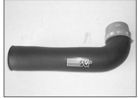
21. Install the silicone hose onto the K&N® intake tube as shown
