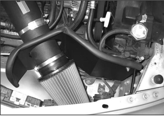
26. Install the K&N® air filter element onto the intake tube and secure with hose clamp.
