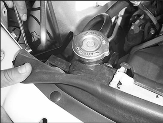
12a. Dakota models only, using the bolt removed in the previous step, secure the short "C" bracket (070672) to the core support.
