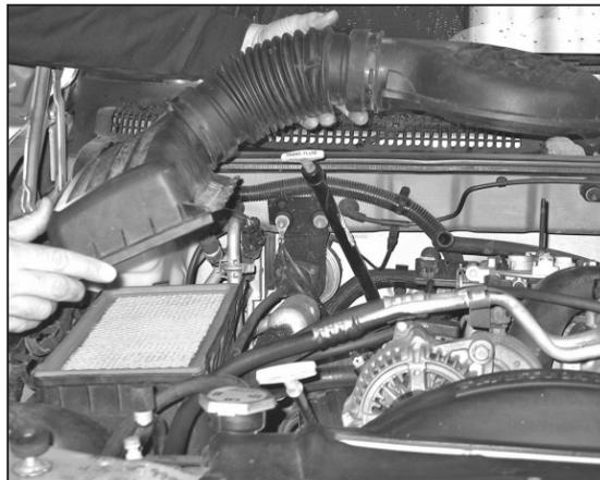
5. Remove the intake plenum and airbox.
