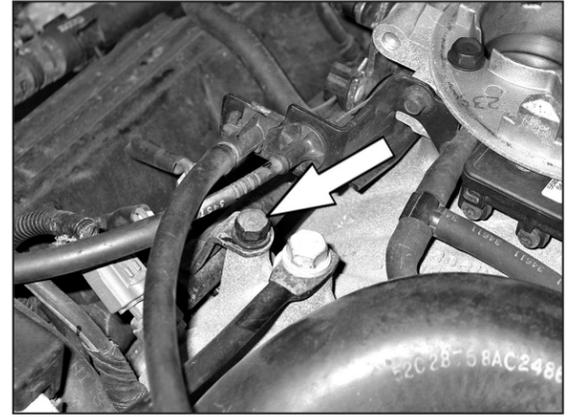
18. Loosen and remove the bolt that retains the fuel rail bracket.
