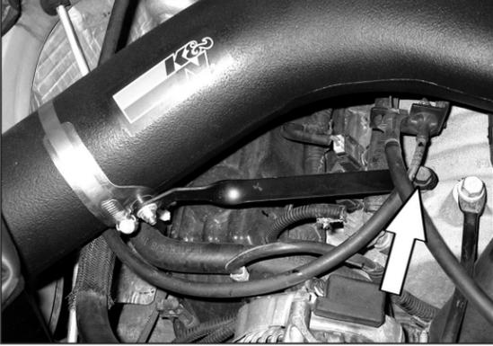
24. Secure the saddle bracket to the intake tube with the provided hose clamp as shown, then tighten the bolt at the fuel rail (see arrow). Position the heat shield for best fit and clearance.
