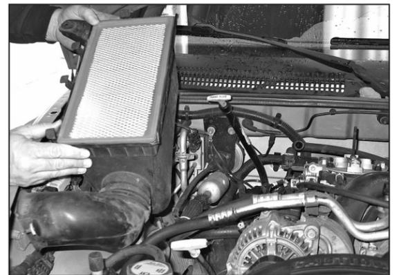
8. Pull firmly upward on the airbox base and remove.
