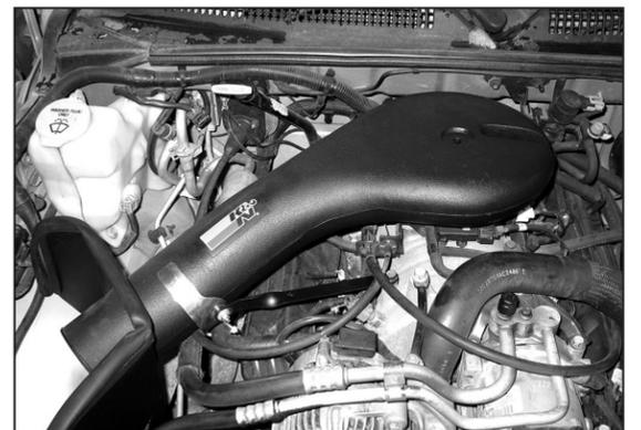
22. Slide the intake tube through the hole in the heat shield as shown.
