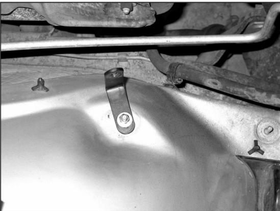
13. Secure the long "L" bracket (070662) to the airbox mounting stud.
