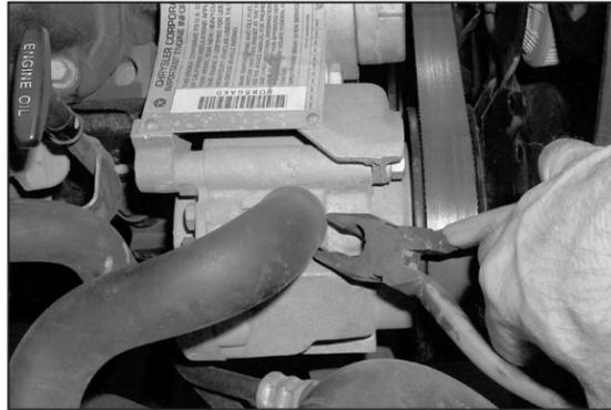
15. On vehicles that come equipped with an air injection pump, release spring clamp that secures the air pump intake hose.
