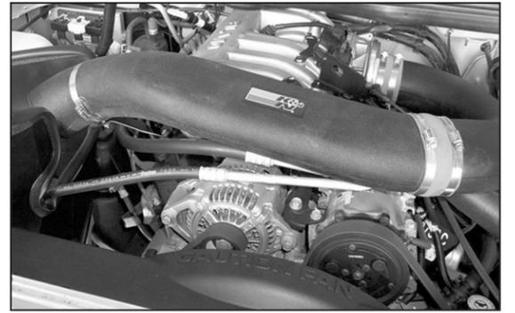
31. Install the second intake tube into silicone hose and then secure the intake tube to saddle bracket.
