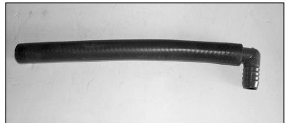
32. On vehicles that come equipped with an air injection pump, install the 90 degree fitting into the vent line as shown.
