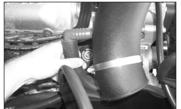
32b. Mark the intake tube where the 90 degree fitting lines up with the intake tube then remove the intake tube from vehicle
