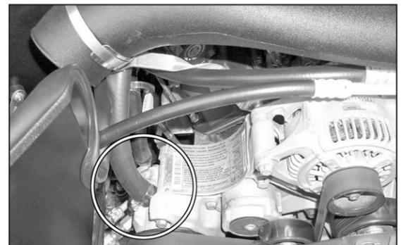
32a. Connect the silicone hose onto the air pump with the provided hose clamp as shown.
