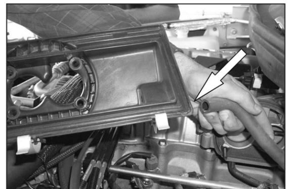
6. Disconnect crank case vent from air box base as shown. Then remove air box from vehicle.
