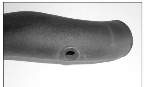
32c. Use a 1-1/4" hole saw and drill a hole where the intake tube was marked in the previous step. Then install the provided grommet as shown.
