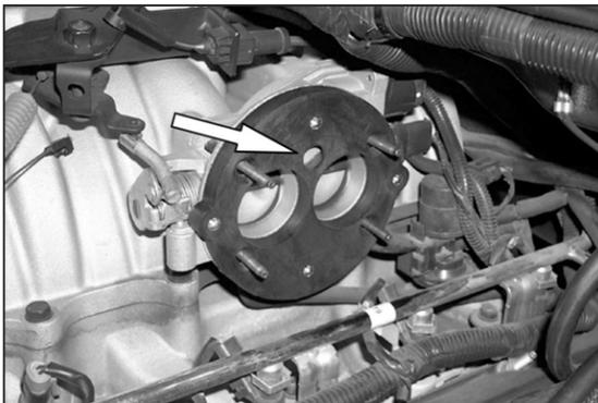
11. Install adapter base plate as shown.
