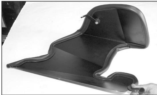
25. Install edge trim onto heat shield as shown. Trim if needed.
