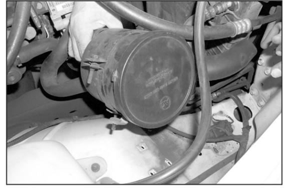
15d. Remove the three 7/16" nuts that retain the air pump muffler. Then pull up to remove the mounting studs from inner fender apron.
