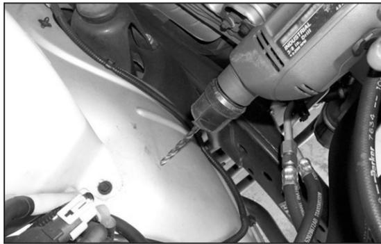
24. Remove heat shield assembly, then drill a 1/4" hole on the spot previously marked.
