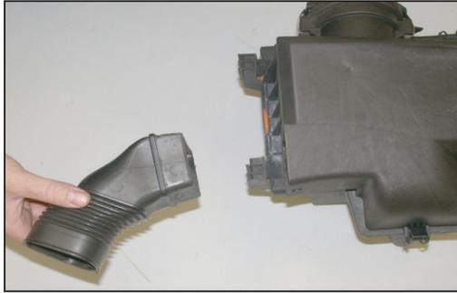
14. Remove the factory fresh air hose from the air box as shown.
