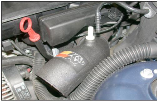
13. Install the K&N® intake tube into the factory lower intake hose and secure with the factory hose clamp.
