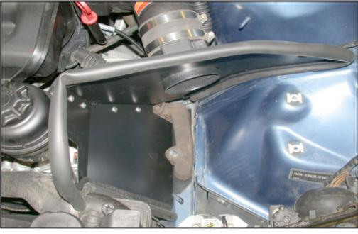
24. Reinstall the lower rubber air box locator removed in step #11 and re-secure the heater hose.
