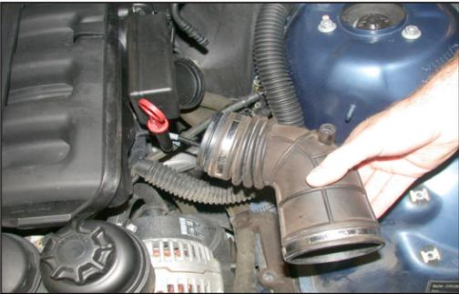
10. Loosen the lower hose clamp and remove the factory upper intake hose from the lower intake hose.
