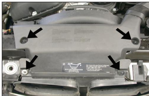
3. Pull up on the four fresh air duct-retaining pins to release them from the radiator core support.
