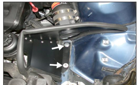
23. Install the heat shield assembly into the vehicle and secure to the lower air box locating studs with the provided hardware as shown. Pass the mass air sensor through the hole in the heat shield.
