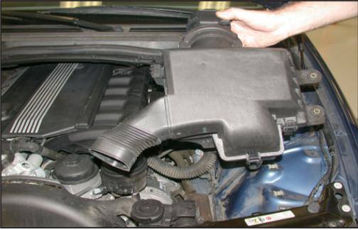
8. Lift up and remove the air box from the vehicle.
