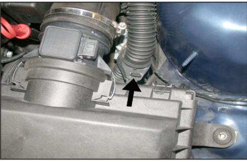
7. Unhook the wiring harness from the rear of the factory air box.
