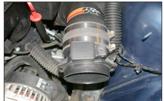
22. Install the mass air sensor assembly onto the K&N® intake tube and secure with the provided hose clamp.
