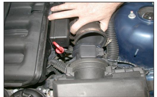
5. Loosen the hose clamp that secures the intake tube to the mass air sensor and then disconnect the intake tube from the mass air sensor as shown.
