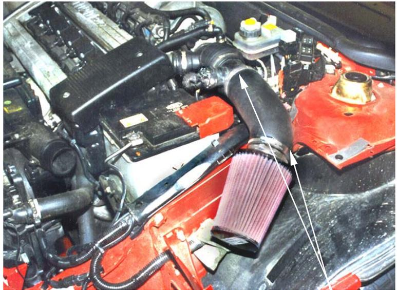
**3.** Fit the metal tube up to the step in the filter base. Do not push beyond the step as this will affect air flow. Tighten the clip until the filter just turns, then give the clip one full turn (360 degrees) **no more. Do not overtighten the clip.**
