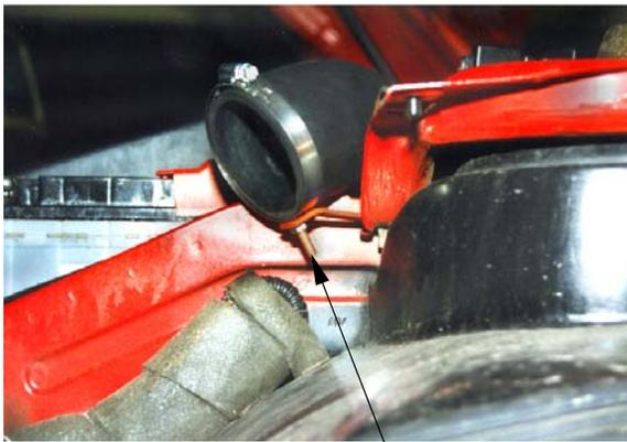
**1.** Fit the new intake hose to the MAS and secure with a hose clip supplied. Do not fully tighten the clip yet.
