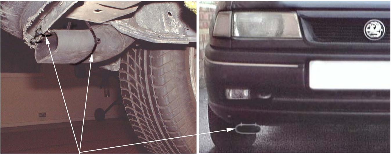
Pierce / drill two 3mm holes in the front bumper trim, secure the new cold air scoop to the front bumper using 2 plastic ties. Insert the flexi cold air hose into the new scoop, secure the scoop to a hole in the cross member with a long plastic tie.
