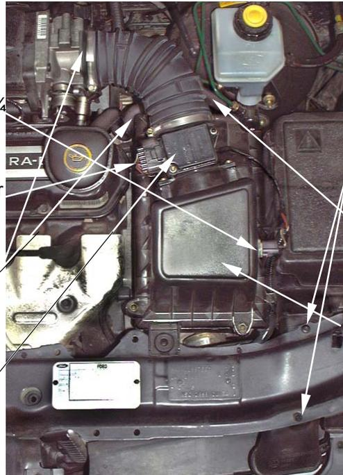
1. Unscrew the air temp sensor 1/4 turn anti clockwise.
