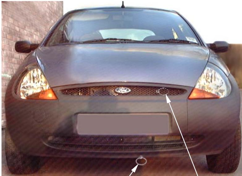
1. Drill / Pierce a 3mm hole in the lower spoiler then pierce a hole in the end of the flexi cold air hose and attach it to the lower skirt using one of the plastic ties provided. Ovalise the end of the cold air hose to increase ground clearance.
