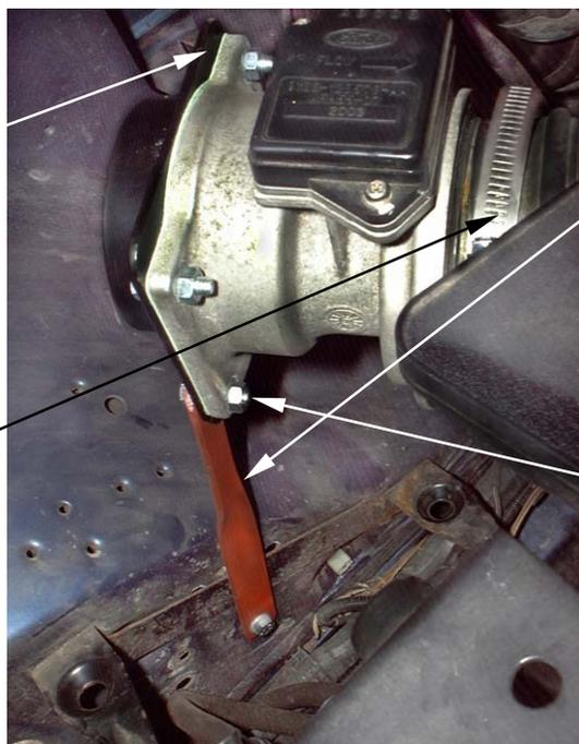
**3.** Attach the new mounting bracket to the inner wing using a short screw, large flat washer, small flat washer, spring washer and nut supplied.
