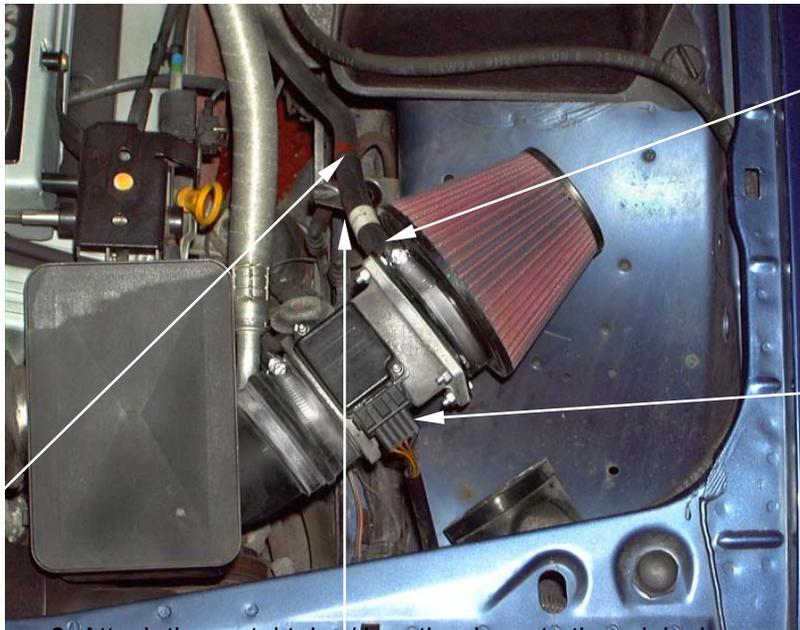
3. Attach the metal tube / breather hose to the original breather hose and secure with the original clip.
