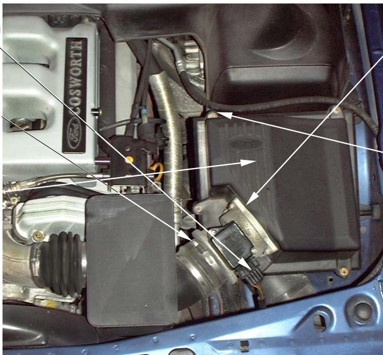
**4.** Separate the MAS from the air box lid by removing the securing screws from inside the lid.
