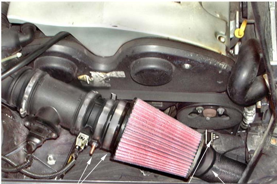
1. Fit the filter onto the metal tube up to the step in the filter base. Do not push in beyond the step as this will affect air flow. Tighten the clip until the filter just turns, then give the clip one full turn (360 degrees) **no more. Do not overtighten the clip.** Fit the tube / filter assembly into the intake hose, rotate the filter until the K&N logo is straight then fully tighten the studded hose clip.
