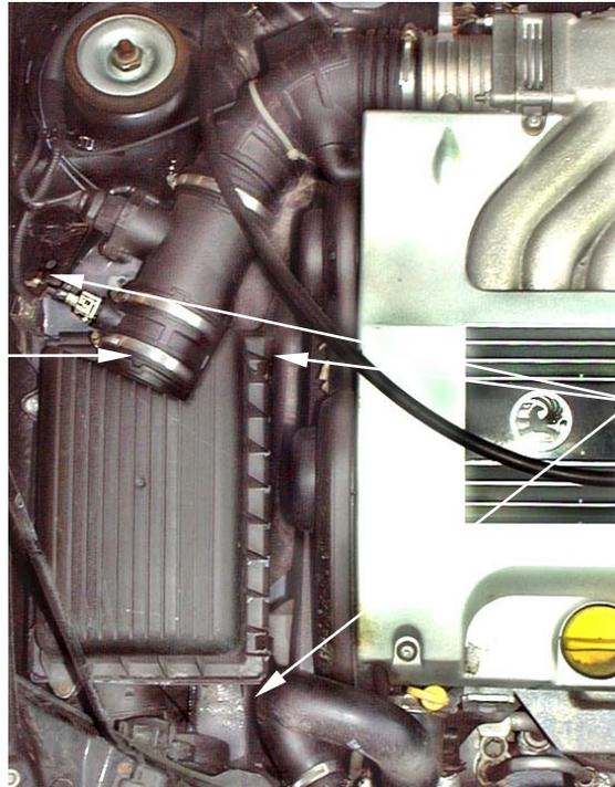
3. Remove the 3 securing nuts from the air box base and lift out the complete assembly
