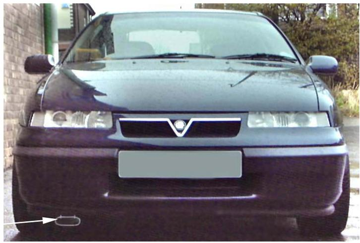
Pierce / drill two 3mm holes in the front bumper trim, secure to the front bumper using 2 plastic ties. Insert the flexi cold air scoop, secure the scoop to a hole in the cross member with
