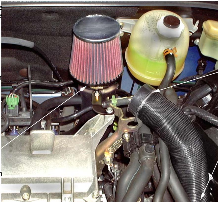
3. Carefully lengthen the flexi cold air feed hose. Attach the end of the hose to the engine lift bracket using a long plastic tie supplied. Position the end of the flexi cold air hose to finish **10cm / 4"** from the filter **no nearer.**
