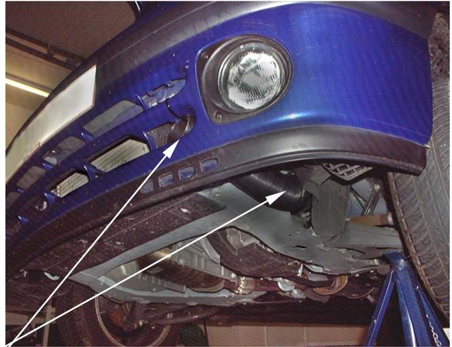
Instructions as per the manufacturer's instructions carefully raise the hose past the side of the arch liner and feed towards the radiator and remove a plastic cover from the side of the radiator. Feed the hose into the front grille area, pierce a 3mm hole in the end of the grille using a plastic tie supplied.
