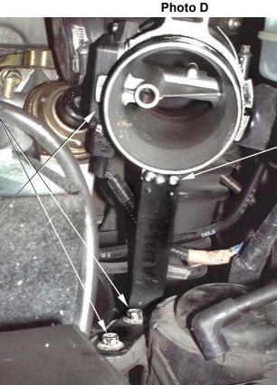
**3.** Attach the MAS to the new mounting bracket.
